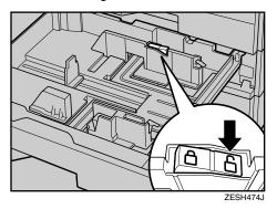
Pushing the green lever of the side guide (①), move the side guide toward you to open it (②).
