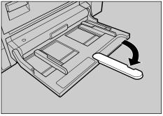
2 Slide the side guides outward (1), and then load paper until it stops with the print side down ((2)).
