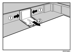
Slide the paper tray into the printer carefully until it stops.
