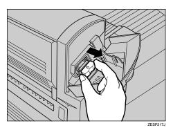
Open the face plate (1) of the cartridge to unlock it.
