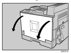
2 Open the right cover of the printer by pushing up the handle.
