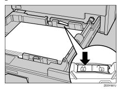
Pinching both sides of the end guide (①), move the end guide toward the paper stack until it stops (②).
