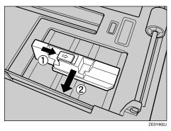
Pinching both sides of the end guide (1), move the end guide in the direction of the arrow (2) to open it.
