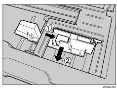
Pinching both sides of the end guide (1), move the end guide in the direction of the arrow (2) to open it.
