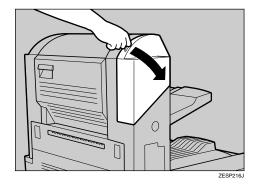
Remove the cartridge by pulling the green knob in the direction of the arrow.
