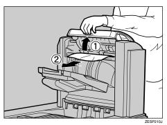
If you still cannot remove the misfed paper, see inside the Interchange Unit. See p.59 "Removing Misfed Paper from the Interchange Unit".
