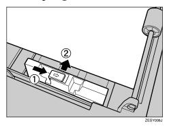
Onfirm that the paper is fixed in place, and then lock the side guides.
