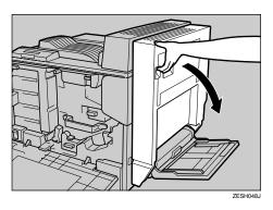
Open the right cover of the printer by pushing up the handle.
