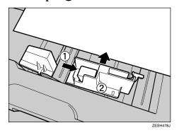
Confirm that the paper is fixed in place, and then lock the side guides.
