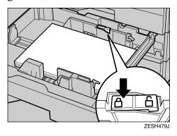
Pinching both sides of the end guide (①), move the end guide toward the paper stack until it stops (②).
