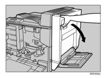
**5** Open the right cover of the printer by pushing up the handle.
