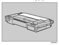
Set the new development unit by aligning the guides, pushing towards direction (①), and then inserting slowly until it stops (②).
