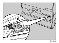
Wipe the rubber of the paper feed rollers with a well-wrung wet cloth.
