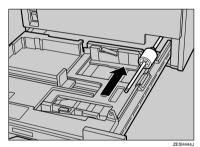
Wipe the rubber of the paper feed roller and the white part of the friction pad with a well-wrung wet cloth.
