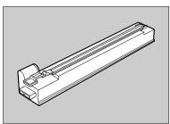
Remove the used waste toner bottle 1 slowly by pinching the lever and then pulling the handle.
