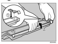
Holding the green part at the center of the fuser oil unit, align the shaft of the fuser oil unit with the metal holder of the fusing unit (1), and then set the fusing oil unit firmly by rotating it to the direction of the arrow (2).
