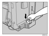
In the next step, replace the photoconductor unit.
