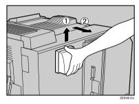
Remove the dustproof filter slowly by holding the tab on the bottom, and then put it in the bag that the new filter came in.
