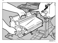
By holding the beige handle of the photoconductor unit as shown in the illustration, tighten the screw that you released in step to tighten the stopper.
