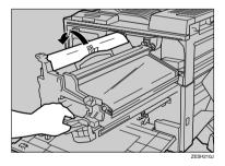
By holding the beige handle of the photoconductor unit, insert the unit slowly until it stops.
