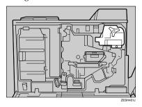
Release the green screw that is fastening the fusing unit.
