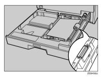
2 Lower the base panel by pushing "Push". When paper is loaded in the tray, push down on the paper.
