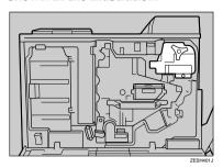
5 Release the green screw that is fastening the fusing unit.
