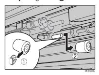
Take out the new paper feed rollers (A), (B) and (C).
