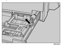
Set the new friction pad by inserting its projection to the hole until it clicks.
