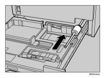
Remove the friction pad by holding its sides.
