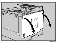
2 Open the green toner cartridge cover by pinching the lever and then pulling the handle.
