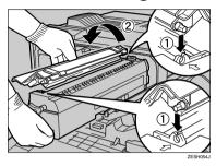
Remove the two red fittings along with the tapes from the fuser oil unit.
