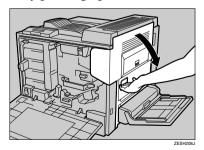
The fuser oil unit is placed on the fusing unit shown in the illustration.
