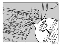
Remove the paper feed roller from the bar by pulling it out (②) while pushing its stopper outwards (①).
