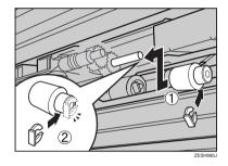
Set the new paper feed roller (A) by inserting it on the bar (①) until the stopper clicks into place.
