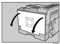
Waste toner bottle 2 is installed as shown in the illustration.
