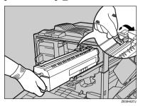
Holding the handle, insert the fusing unit slowly until it stops.
