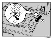
Set the new paper feed roller on the bar by pushing it through with the stopper (1) facing towards you.
