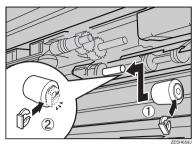
Set the new paper feed roller (B) by inserting it on the bar (1), and then placing the stopper on it (2).
