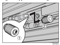
Remove the paper feed roller (B) by removing its stopper (1), and then pulling it out (2).
