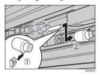
Remove the paper feed roller (C) by removing its stopper (①), and then pulling it out (②).
