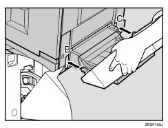
Align the projections and dents on the Duplex Unit and the printer, and then slide the Duplex Unit to the right until it clicks into place.
