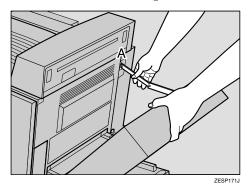
Connect the bar firmly as shown in the illustration.
