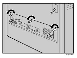
The screws cannot be fully removed.
