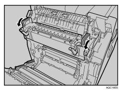
**B** Pull out the fusing unit.
