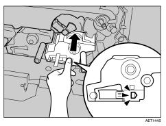
🕑 Hold the photo conductor unit firmly in place, and then pull out the tape.
