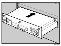
Push on the area of the controller board that is marked "PUSH". Push in the controller board until it can go no further.
