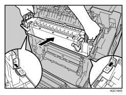
**O** Push the fusing unit carefully in, until it stops. Then, pull up the fixing lever.
