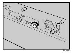
Carefully insert the Data Overwrite Security unit, until the card clicks into place.
