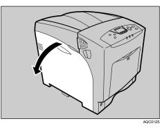
**1** Turn the two green levers of the inner cover anticlockwise (1), and then slowly open the inner cover (2).
