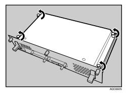
The screws cannot be fully removed.
