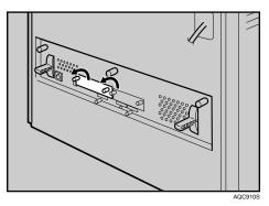
The removed cover is not used when installing the interface unit.
