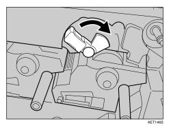
Close the inner cover. Lock the inner cover by pressing in (1) and then turning the two green levers clockwise (2).
