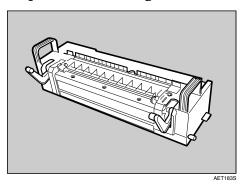
**5** Align the new fusing unit with the left and right rails.
