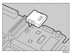
**B** Make sure that User Account Enhance Unit is firmly connected to the controller board.
