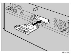
Confirm that the 1284 interface board is firmly connected to the controller board.
