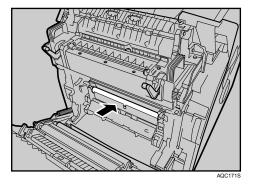
Clean the registration roller by applying a soft damp cloth while turning it.
