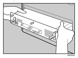
**5** Place the controller board on a flat surface. Loosen the five screws to remove the cover
