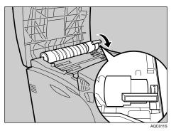
Do not repeatedly install and remove toner cartridges. Doing so results in toner leak.
