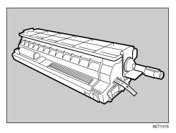
B Remove the protecting cover. Do not remove the tape yet.
