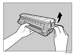
Check the installation position of the photo conductor unit. Install the unit where the colored labels correspond.
