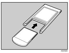
**2** With the label side facing left, slowly push the card adapter into the interface unit until it stops.
