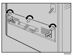
The screws cannot be fully removed.
