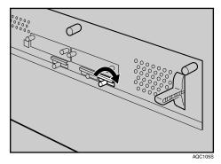
Carefully insert the Camera Direct Print card, until the card clicks into place.
