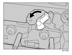
**6** Pull out the handle of the transfer unit. Grasp the handle and the green lever firmly, and then slowly pull out the transfer unit, until the green line marked on the upper surface of the unit appears.
