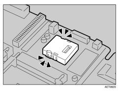
**9** Fasten the four screws to attach the cover.
