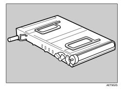
Hold both upper handles, and then slide the transfer unit along the guide rails into the printer.
