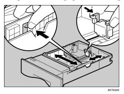
**3** Slide the green switch on the front of the tray to the type of paper to be loaded. When loading paper of 75 g/m<sup>2</sup>, 20 lb., or thicker, slide the switch to the right.
