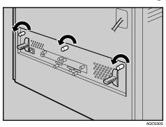
The screws cannot be fully removed.
