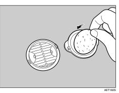
**5** Reattach the dustproof filter covers to the printer one at a time.
