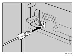
If the gigabit ethernet board is attached, connect the ethernet cable to the board.
