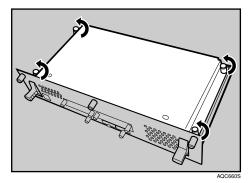
The screws cannot be fully removed.
