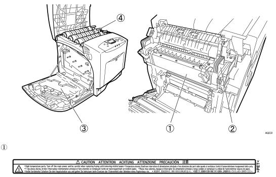
High temperature parts. Turn off the main power and be careful when replacing fusing unit/removing misfed paper.
