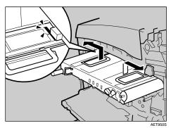
Grasp the raised up handles with both hands, and then pull the transfer unit completely out.
