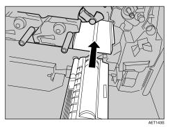
Take care that nothing comes into contact with the surface of the photo conductor unit.
