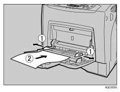
Adjust the side guides to fit the paper width.
