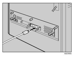
The printer's ethernet and USB ports are not available when the gigabit ethernet board is attached to the printer.
