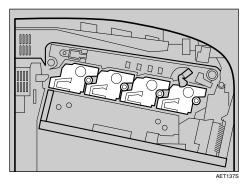
Remove the photo conductor unit you want to replace. Turn the green lever counterclockwise to unlock the unit. (The black photo conductor unit is used in this example.)
