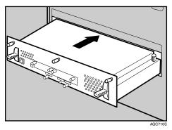
Push only on the area of the controller board that is marked "PUSH". Push in the controller board until it can go no further.
