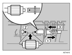
Check the green lock lever secures the roller correctly by making sure the new roller rotates smoothly.
