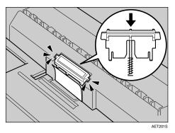
After pushing down the friction pad, check it is properly installed by pressing it lightly. If it is properly installed, it will spring back up.
