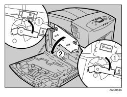
The photo conductor units are installed as shown. From the right, the units are attached in the order of black (K), magenta (M), cyan (C), and yellow (Y).
