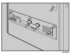
Attach the card to the card adapter. Attach them so that the label on both the card and adapter is facing up.
