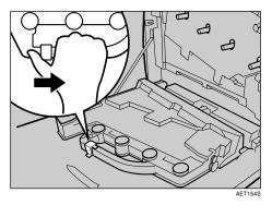
**E** Lift the waste toner bottle with the seal still attached, and then remove the waste toner bottle from the left cover.
