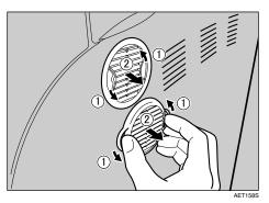
Place the removed dustproof filter cover down on a stable and level surface.
