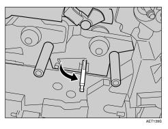
**6** Hook your finger through the ring pull handle, and then slowly pull out the photo conductor unit. When you have pulled the unit half way out, support the photo conductor unit using your other hand, and then pull the unit completely out.
