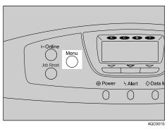
**2** Select [Paper Input] using [▼] or [▲], and then press the [OK] key.
