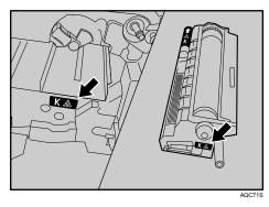
Install the photo conductor unit with the tape still attached. Align the tip of the photo conductor unit with the opening, and then slowly insert the unit, until it stops.
