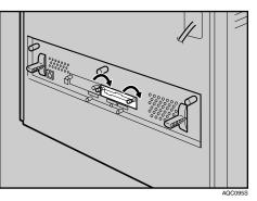
**1** Attach the antenna to the card with the label facing down and the uneven side of the antenna facing up.
