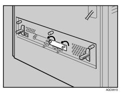
The removed cover is not used when installing the 1284 interface board.
