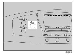
**2** Select [Host Interface] using [▼] or [▲], and then press the [OK] key.
