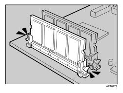
**1** When replacing the default SDRAM module, press down the levers on both sides (1) to remove the default module (2).
