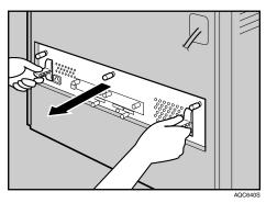
Using both hands, slide the controller board completely out.
