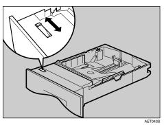
Load the new paper stack print side up, making sure the paper is flush against the paper guides. Adjust the paper guides to close any gaps.
