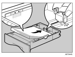
**5** Lift the front of the paper tray (Tray 1), and slowly slide the paper tray back in, until it stops. Make sure the tray is fully inserted to prevent a paper misfeed.
