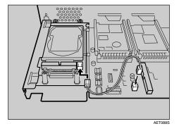
**2** Connect the flat cable to the hard disk drive and the controller board. Connect the blue end of the flat cable to the controller board.
