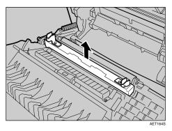
Insert the new transfer roller by placing its underside edge into the grooves shown in the illustration.
