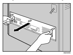
Using both hands, slide the controller board completely out.
