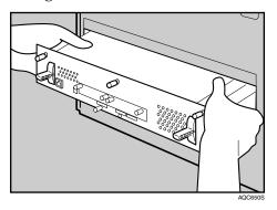
Place the controller board on a flat surface, and then loosen the four screws to remove the cover.
