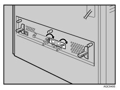
Check the Gigabit ethernet board is connected firmly to the controller board.
