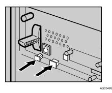
Loosen the two screws and remove the cover of the Gigabit ethernet board installation unit.
