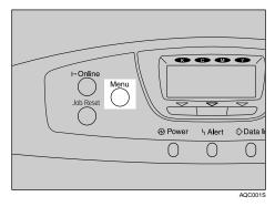
**2** Select [Paper Input] using [▼] or [▲], and then press the [OK] key.
