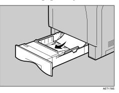
Push in the paper tray. Make sure the tray is securely inserted to avoid paper jams.
