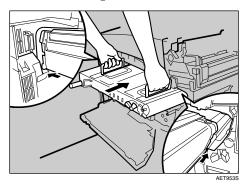
The upper handles must be raised to insert the unit.
