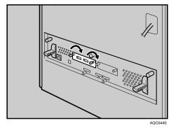
Check the USB host interface board is inserted firmly to the controller board.
