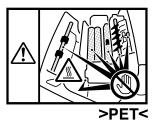
The inside of this printer becomes very hot. Do not touch parts labelled " $\Delta$ " (indicating a hot surface). Touching these parts will result in burns.
