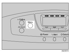
**2** Select [Maintenance] using [▼] or [▲], and then press the [OK] key.
