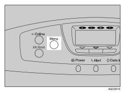
**2** Select [Host Interface] using [▼] or [▲], and then press the [OK] key.
