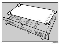
Align the controller board with the left and right rails, and then push it carefully in, until it stops.
