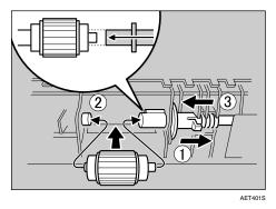
Confirm that the green lock lever secures the roller correctly by confirming that the roller rotates smoothly.
