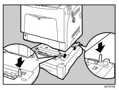
When installing two paper feed units, connect the two units first using the same procedure below before connecting the units to the printer.
