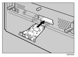
**6** Tighten the two screws to secure the Gigabit ethernet board.
