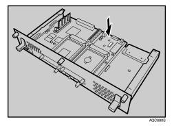
**2** Align the notch of User Account Enhance Unit, and then insert it into the controller board, pressing it down until it clicks into place.
