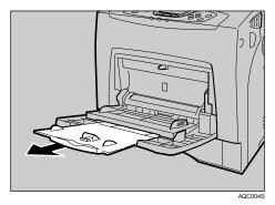
**3** Slide the side guides outward, and then load paper print side down, until it stops.
