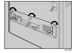
**B** Fasten the controller board to the printer using the three screws.
