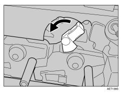
**5** Pull out the ring pull handle of the photo conductor unit.
