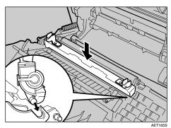
**5** Secure the transfer roller using the green fastening clips mentioned in step **2**.
