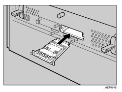
**•** Tighten the two screws to secure the interface unit.
