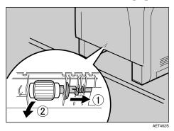
**2** While sliding the green lock lever to the right (1), set the new roller (2). Then, return the green lock lever to its original position (3).
