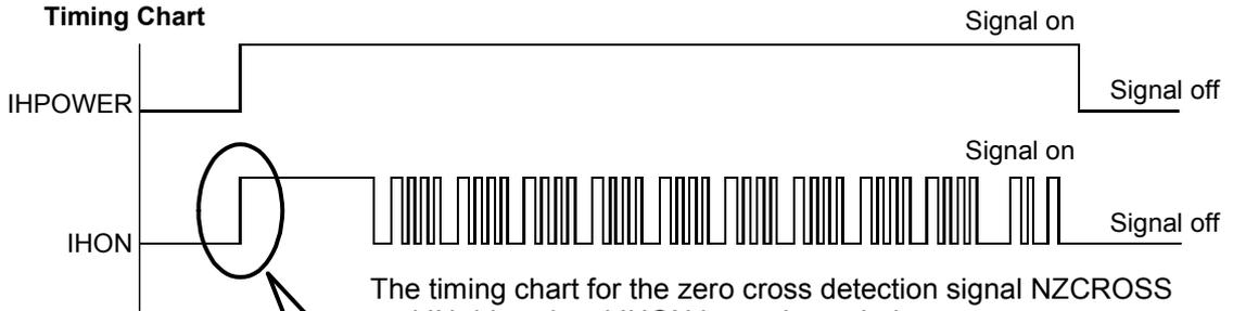
The timing chart for the zero cross detection signal NZCROSS and IH drive signal IHON is as shown below.
