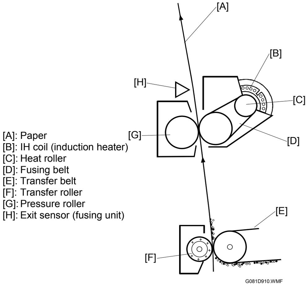
After the toner image has been applied to the paper [A], it passes through the fusing unit. The fusing unit contains the heat roller [C]. The IH coil [B] heats the heat roller. The heat roller heats the fusing belt [D] to melt the toner on the paper. The paper is pressed between the fusing belt and the pressure roller [G], and melted toner bonds to the paper.
