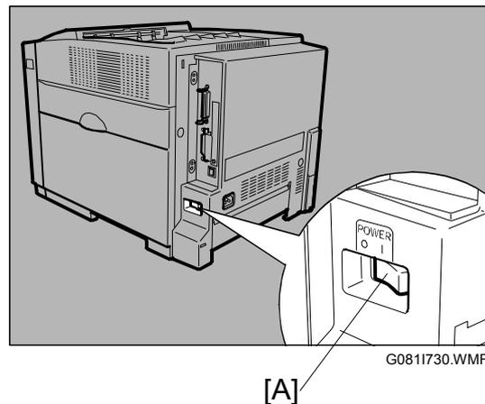
2. Attach the power cord to the socket on the back of the printer.
