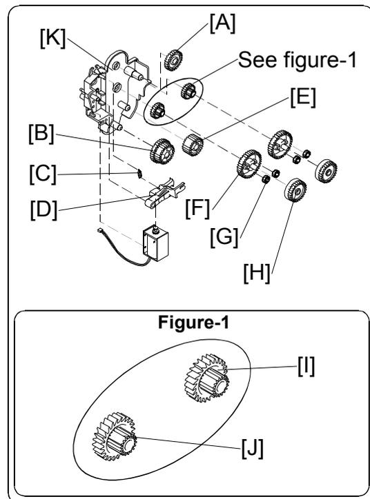
**CAUTION:** The rotation switching gear [I] differs from the other gear [J] in the direction of the gear teeth (see Figure-1).
