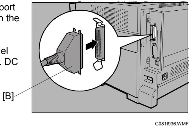
4. Attach the other end of the parallel cable to the port of the computer. Secure the cable.
