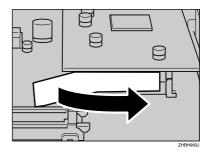
Lift the end of USB2.0 Interface Unit (①), and then remove it from the controller board (②).
