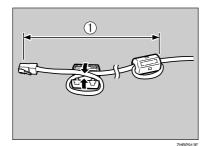
Attach the network interface cable to the jack on the Network In-
