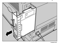
The Printer Hard Disk is to be installed to the position shown in the illustration.
