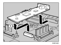
Attach the Bluetooth Interface Unit. Insert the end of the Bluetooth Interface Unit to the opening (1), and then push down until it clicks (2).
