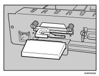
Adjust the Bluetooth module to the slot, and then insert vertically.
