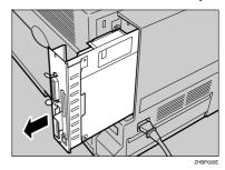
There are two slots for the Memory Unit. Use the available slot (the one in the front in the illustration ②) to install an optional Memory Unit
