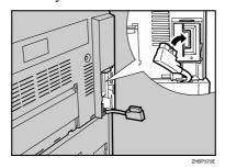
Close the connector cover of the printer.
