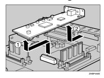
8 Attach the 1394 Interface Unit to the controller board. Insert the end of the 1394 Interface Unit into the opening (①), and then push down until it clicks (②).
