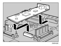
8 Attach the 802.11b Interface Unit. Insert the end of the 802.11b Interface Unit to the opening (1), and then push down until it clicks (2).
