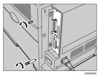
The removed screws will be used in step **11** to fasten the controller board.
