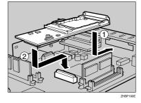
Confirm that the Bluetooth Interface Unit is firmly connected to the controller board.
