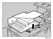
Confirm that the User Account Enhance Unit is firmly connected to the controller board.
