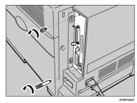
The removed screws will be used in step ① to fasten the controller board.
