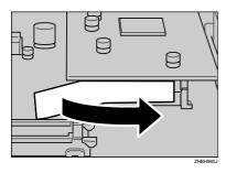
**7** Lift the end of USB2.0 Interface Unit (1), and then remove it from the controller board (2).
