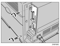
The removed screws will be used in step 3 to fasten the controller board.
