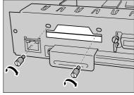
Attach the antenna to the card with the label facing down and the uneven side of the antenna facing up.
