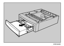
5 Remove the adhesive tape and packing material.
