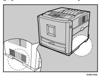
8 Align the printer to the two upright pins on the Paper Feed Unit and then lower it slowly.
