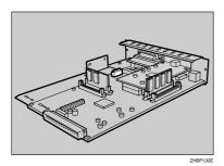
5 Set the User Account Enhance Unit on the controller board in the direction shown in the illustration.
