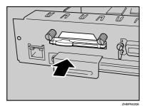
Attach the antenna cap over the antenna.
