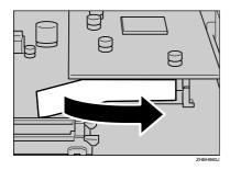
Lift the end of USB2.0 Interface Unit (1), and then remove it from the controller board (2).
