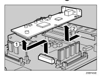
8 Attach the Network Interface Board. Insert the end of the Network Interface Board to the opening (1), and then push down until it clicks (2).
