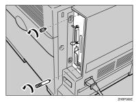
The removed screws will be used in step 3 to fasten the controller board.
