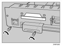
Insert the card slowly into the Bluetooth Interface Unit with its side labeled "INSERT" facing up until it stops.
