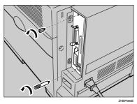
The removed screws will be used in step **7** to fasten the controller board.
