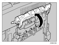
Unlock the waste toner bottle by sliding the green arrow to the position as shown.
