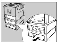
3 Slide the paper tray completely into the printer.
