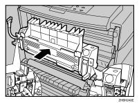
8 Insert the fusing unit until it clicks, and then check that the unit is locked.
