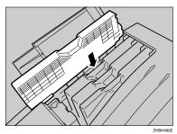
Insert the toner cartridge in the direction of the arrow.
