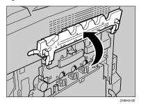
**5** Remove the photo conductor unit.
