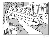
Push the front of the photo conductor unit slowly, sliding the unit on the cover and into the machine until it stops.
