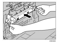
Turn the green screws on the left and right in the direction of the arrows to tighten them.
