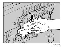
2 Pull out the photo conductor unit slowly until it stops.
