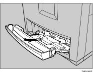
3 Slide the side guides outward (), and then load paper until it stops with the print side down (2).
