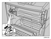
Push the green release buttons on the left and right outwards to unlock the fusing unit.
