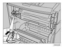
Turn the green part in the direction of the arrow, and then remove the transfer roller.
