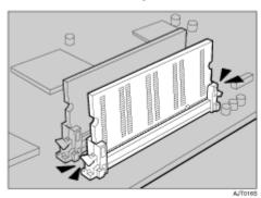
When replacing the default SDRAM module, press down the levers on both sides (1) to remove the default module (2).
