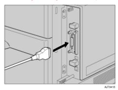
Securely attach the other end of the parallel cable to your computer's parallel port. Secure the cable.
