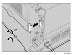
The removed cover and two screws are not used when installing the 1394 interface board.
