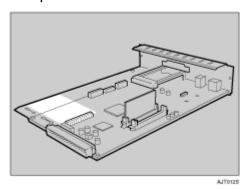
Insert the printer hard disk by aligning it with the controller board slot. Slide it in the direction of the arrow, and then connect it to the connector on the controller board.
