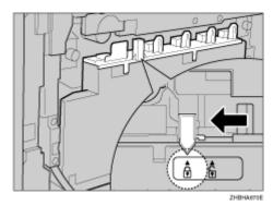
Pull out the green levers on the left and right that are securing the inner cover, and then unlock.
