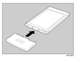
With the antenna and indented end toward the printer front cover, slowly insert the interface card until it stops.
