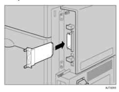
**5** Tighten the two screws to secure the interface unit.
