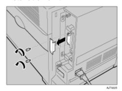
The removed cover and two screws are not used when installing the 1284 interface board.
