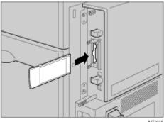
Holding the antenna cap with the two cut off corners toward the printer front cover, fit the cap over the card.
