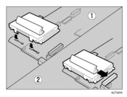
2 Secure the printer hard disk using the supplied screw.
