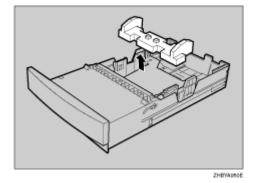
Slide the paper tray fully into the paper feed unit.
