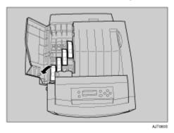
Check the toner color and location are correct, and then carefully insert the toner cartridge vertically.
