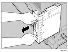
There are two slots for the Memory Unit. Use the available slot to install an optional Memory Unit
