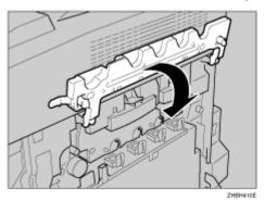
Push the left and right edge of the inner cover to secure it.
