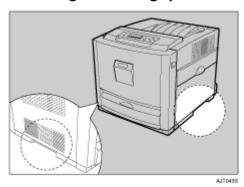
Align the printer with the two upright pins on the paper feed unit, and then lower it slowly.
