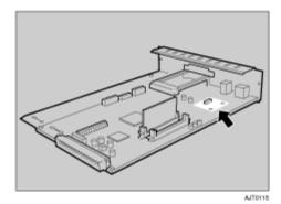
Align the notch of the user account enhance unit, and then insert it into the controller board, pressing it down until it clicks into place.
