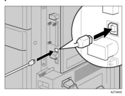
2 Connect the opposite end's flat connector to devices such as your computer's USB interface, or a USB hub.
