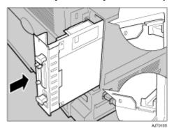
Hold the machine with one hand, and then push the lower handle of the controller board with the palm of your other hand, until it stops.
