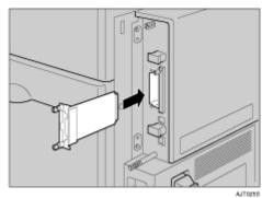
**5** Tighten the two screws to secure the interface unit.
