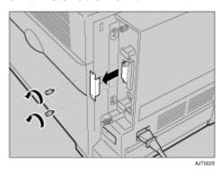
The removed cover and two screws are not used when installing the interface unit.
