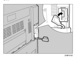
To connect two paper feed units, connect the paper feed unit cable securely to the socket inside the paper feed unit
