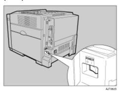
2 Attach the power cord to the socket on the back of the printer.
