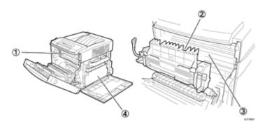
① High temperature parts. Turn off the main power and be careful when replacing fusing unit / removing misfed paper.
