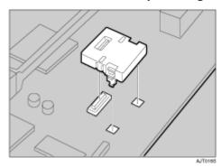
Make sure that the user account enhance unit is firmly connected to the controller board.
