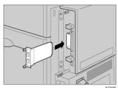
Make sure that the 1394 interface board is firmly connected to the controller board.
