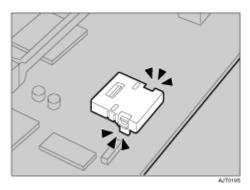
Align the controller board with the top and bottom rails, and then push it carefully in until it stops.
