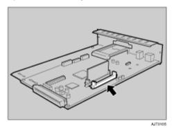
Adjust the notch of the Memory Unit to the slot, and then insert vertically.
