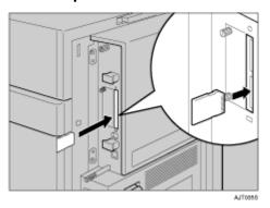
B Reattach the cover over the network data protection unit. Fasten the screw to secure the cover.
