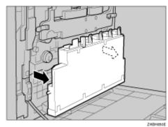
Loosen the green screws on the left and right by turning them the direction of the arrows.
