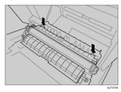
Turn the green part in the direction of the arrow, and then remove the transfer roller.
