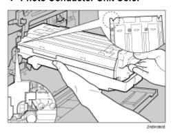
Push the front of the photo conductor unit carefully in sliding the unit from its cover until it stops.
