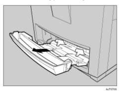
Slide the side guides outward (①), and then insert paper print side down until it stops (②).
