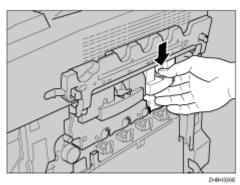
Pull out the photo conductor unit carefully.
