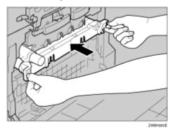
Tighten the green screws on the left and right by turning them the direction of the arrows.
