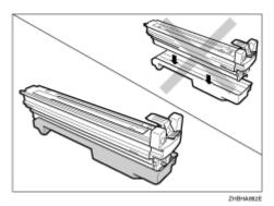
E Check the locations for each Photo Conductor Unit.
