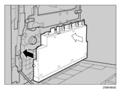
Lock the waste toner bottle by sliding the green arrow to the position shown.
