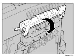
f E Push the left and right edge of the inner cover to secure it.
