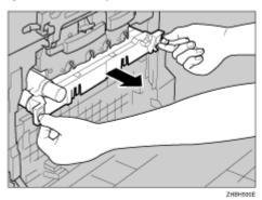
Raise the green cover, hold the transfer belt as shown, and then remove the transfer belt.
