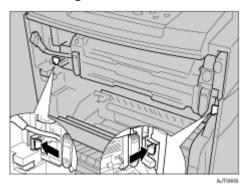
**5** Remove the fusing unit carefully.
