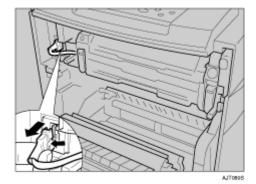
2 Push the green release buttons on the left and right outwards to unlock the fusing unit.
