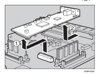
6 Attach the Network Interface Board. Insert the end of the Network Interface Board to the opening (①), and then push down until it clicks (②).
