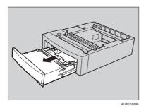
Remove the adhesive tape and packing material.
