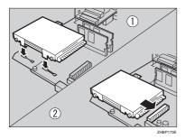
**6** Fasten the Printer Hard Disk using the supplied screw.
