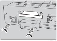
8 Insert the card slowly into the Bluetooth Interface Unit with its side labeled "INSERT" facing up until it stops.
