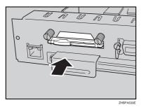
Attach the antenna cap over the antenna.
