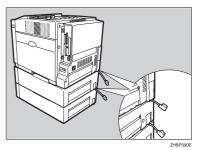
Open the connector cover of the printer.
