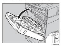
4 Hold the Duplex Unit as shown in the illustration, and then insert it into the inside of the front cover.
