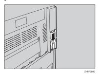
To connect two Paper Feed Units, connect the paper feed unit cable to the socket inside the Paper Feed Unit securely, and then close the connector cover.
