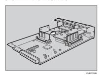
Set the User Account Enhance Unit on the controller board in the direction shown in the illustration.
