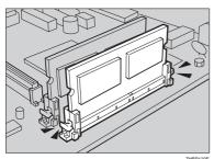
6 Align the controller board to the top and bottom rails, and then push in slowly until it stops.
