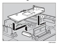
Confirm that the Network Interface Board is firmly connected to the controller board.
