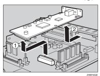
6 Attach the Bluetooth Interface Unit. Insert the end of the Bluetooth Interface Unit to the opening (1), and then push down until it clicks (2).
