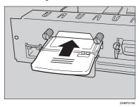
Align the controller board to the top and bottom rails, and then push in slowly until it stops.
