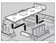
6 Attach the 802.11b Interface Unit. Insert the end of the 802.11b Interface Unit to the opening (①), and then push down until it clicks (②).
