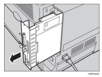
The User Account Enhance Unit is to be installed to the position shown in the illustration.
