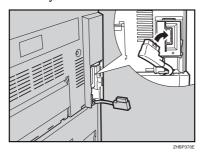
Close the connector cover of the printer.
