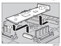
6 Attach the 1394 Interface Unit to the controller board. Insert the end of the 1394 Interface Unit into the opening (①), and then push down until it clicks (②).
