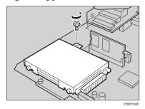
Align the controller board to the top and bottom rails, and then push in slowly until it stops.
