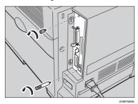
The removed screws will be used in step **7** to fasten the controller board.
