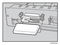
Adjust the Bluetooth module to the slot, and then insert vertically.
