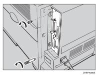
The removed screws will be used in step **9** to fasten the controller board.
