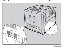
Align the printer to the two upright pins on the Paper Feed Unit and then lower it slowly.
