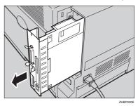
There are two slots for the Memory Unit. Use the available slot (the one in the front in the illustration ②) to install an optional Memory Unit
