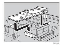
Confirm that the Bluetooth Interface Unit is firmly connected to the controller board.
