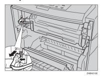
Push the green release buttons on the left and right outwards to unlock the fusing unit.
