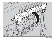
**5** Remove the photo conductor unit.
