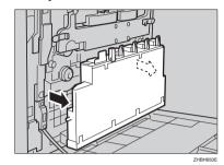
Turn the green screws on the left and right in the direction of the arrows to loosen them.
