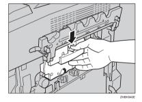
2 Pull out the photo conductor unit slowly until it stops.
