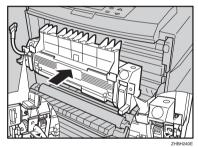
Insert the fusing unit until it clicks, and then check that the unit is locked.
