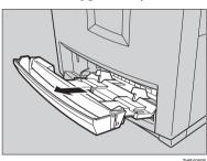
Slide the side guides outward(1), and then load paper until it stops with the print side down (2).
