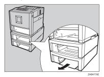
Slide the paper tray completely into the printer.
