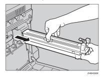
Photo Conductor Unit Type 125 Color
