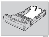
Press "Push", and then adjust the rear guide to the paper size you are using.
