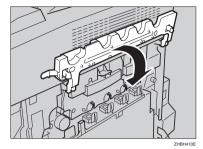
Push the green lever to fasten the inner cover.
