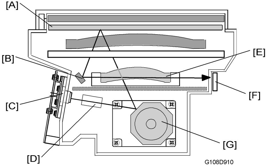
The synchronization detector [F] is on the right side of the optics unit. When emitted from the LD unit [C], the laser travels as follows: cylinder lens [D] → polygon mirror [G] → F-theta lens [E] → first mirror [A] → synchronization mirror [B] → synchronization detector [F].
