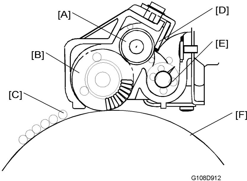
The transfer-belt cleaning unit is on top of the transfer belt [F]. The transfer-belt cleaning unit has these components:
