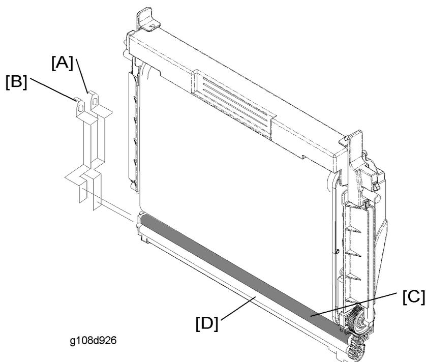
The charge roller [C] gives negative charge to the OPC belt. The cleaning roller [D] cleans the charge roller. The high voltage unit (HVU) gives electrical power to the charge roller and the cleaning roller. The left end of the charge roller is attached to BRV [B] on the HVU. The left end of the cleaning roller is attached to CLV [A] on the HVU.
