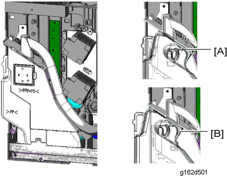
The waste toner holder unit has a shutter. The shutter is pulled by a spring. As a result, the shutter is closed if the waste toner bottle is not installed. This shutter prevents waste toner from falling down inside the machine when the waste toner bottle is removed.
