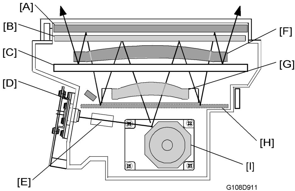
The laser beam moves as follows:
