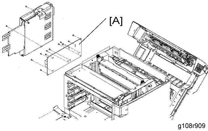
1. Controller box (☛ Power Supply Unit (Direct Current))
