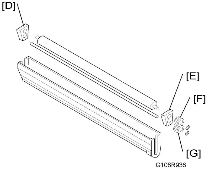
4. Left holder [D] and right holder [E] with the charge roller and the cleaning roller
