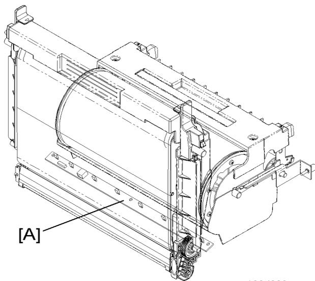
The erase lamp [A] is below the contact point of the OPC belt and the transfer belt. The erase lamp quenches the electrical charge on the OPC belt.
