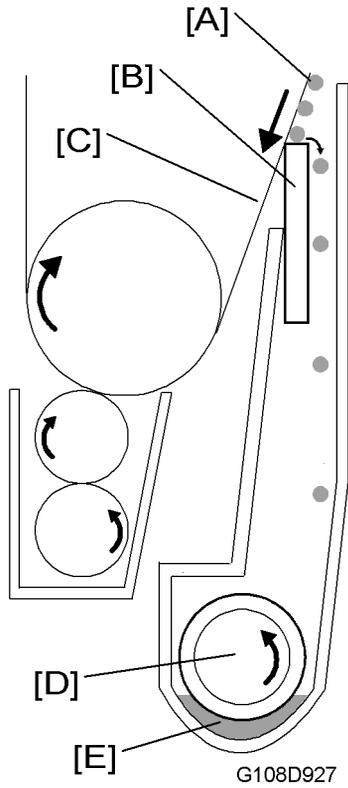
The OPC-belt cleaning blade [B] is near the bottom of the OPC belt [C]. The OPC-belt cleaning blade removes remaining toner [A] from the OPC belt. Removed toner (waste toner) goes into the waste toner duct [E]. The waste toner feeder [D] moves waste toner to the right end of the waste toner duct. At this time waste toner goes into the waste-toner collection unit.
