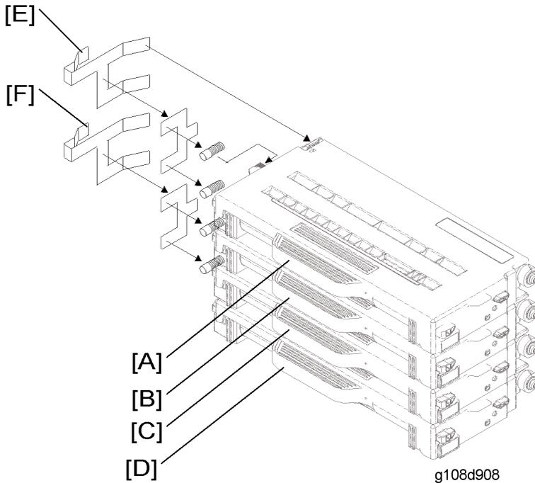
The high voltage unit (HVU) gives development bias to the four development units. The development unit K [A] and the development unit M [B] are attached to DBVKY [E] on the HVU. The development unit Y [C] and the development unit C [D] are attached to DBVMC [F] on the HVU.
