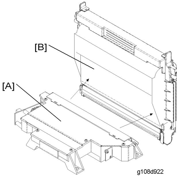
The optical housing unit [A] emits the laser beam and writes latent images on the OPC belt [B].
