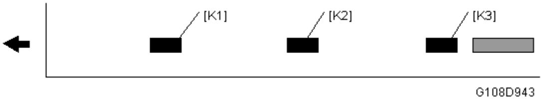
1. The black development unit changes the development bias to make three rectangular images. The first image [K1] is weaker than the second image [K2]. The second image is weaker than the third image [K3].
