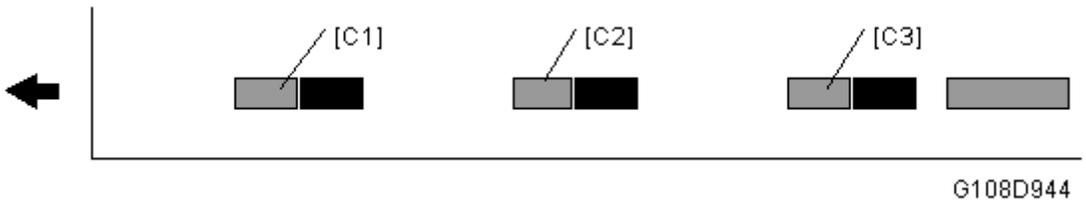
2. The cyan development unit changes the development bias to make three rectangular images. The first image [C1] is weaker than the second image [C2]. The second image is weaker than the third image [C3].
