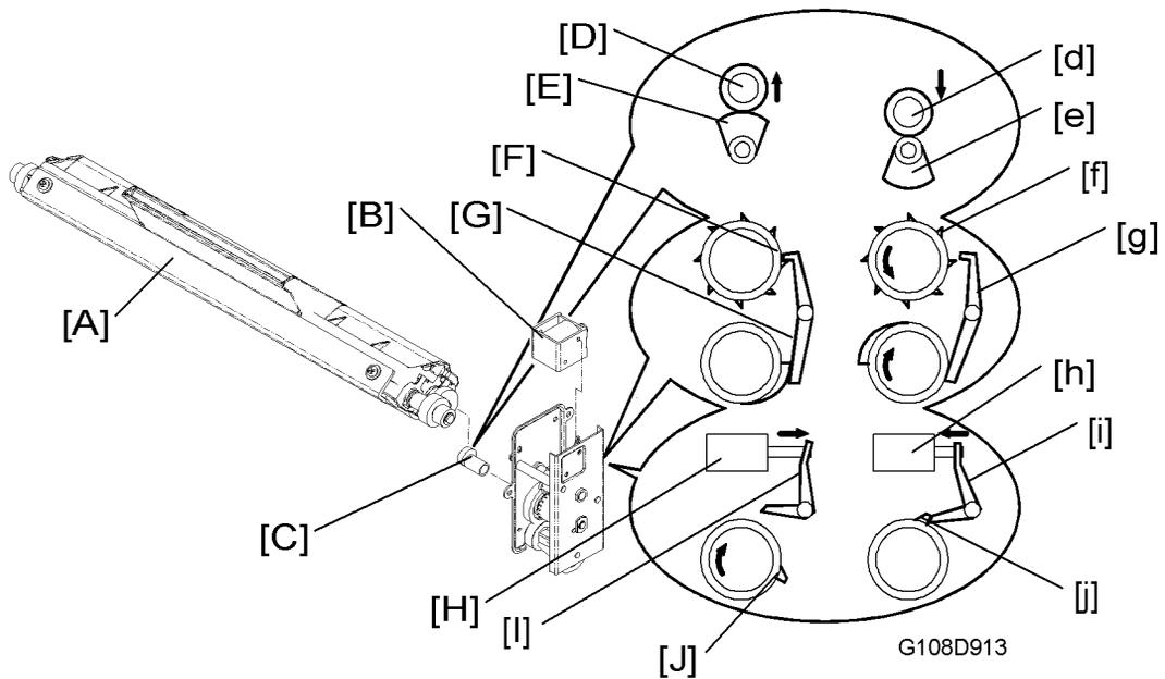
The transfer-belt cleaning unit [A] stays away from the transfer belt when not cleaning the transfer belt. The transfer-belt cleaning unit stays in contact with the transfer belt when it cleans it. These components do this procedure:
