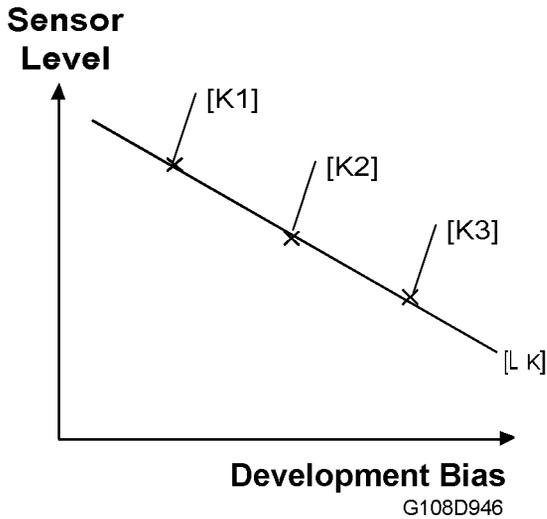
The controller makes these linear equations to adjust the development bias for each color:
