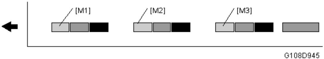
3. The magenta development unit changes the development bias to make three rectangular images. The first image [M1] is weaker than the second image [M2]. The second image is weaker than the third image [M3].
