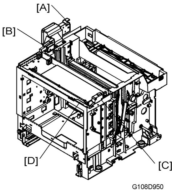
The printer has three safety switches [A][B][C]. They all go on when these covers are closed:
