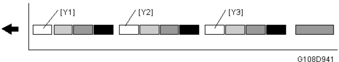
4. The yellow development unit changes the development bias to make three rectangular images. The first image [Y1] is weaker than the second image [Y2]. The second image is weaker than the third image [Y3].
