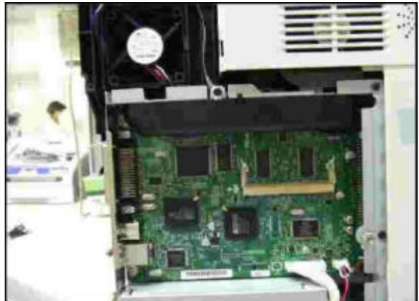
4. Remove the black hook of the harness cover, and then remove the harness cover.
