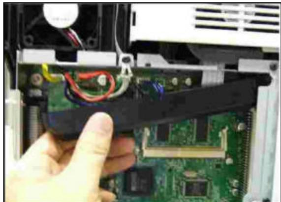
5. Remove the two connectors of the ADF harness.
