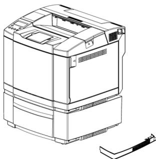
**Hook the pivot at the left back of the paper feeder and turn the left cover around the pivot and fit it on.**
