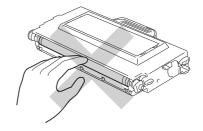
Put in the new toner cartridge by positioning it in the guide. Slide it gently into the machine. Do not try to push or lock the new toner cartridge in; it must rest loosely in the guide rails and will automatically be positioned properly when the front cover is closed. Note that each colour cartridge is individually keyed to prevent improper installation. Match each cartridge colour label to the same colour label on the machine.
