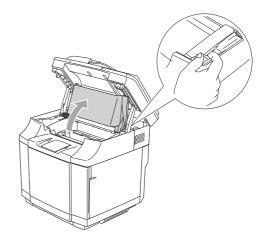
To release the lock, push the green belt cartridge lock levers on both sides inwards.
