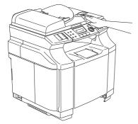
3 Remove any paper that is stuck inside the paper tray.
