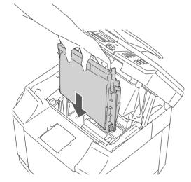
**5** Lock the belt cartridge lock levers.
