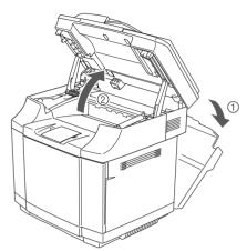
Pull out the protective parts from both sides of the fusing unit.
