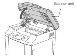
2 Lift the Inside cover so that it latches under the scanner unit.
