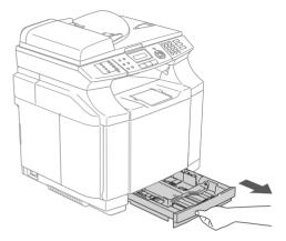
While pressing the paper guide release lever, slide the adjusters to fit the paper size.
