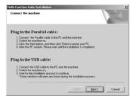
DO NOT plug in the power cord before connecting the parallel Caution interface cable. It may cause damage to your machine.
