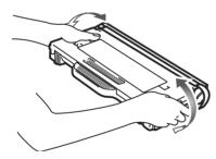
Pull off the tape labelled REMOVE, and then remove the orange protective cover.
