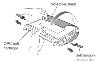
4 Put the OPC belt cartridge into the machine guides with the flat side facing you.
