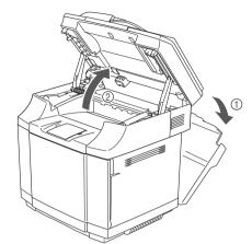
2 Pull out the protective parts from both sides of the fusing unit.
