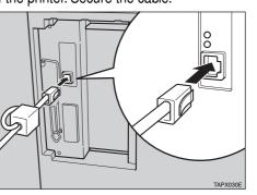
Connect the other side of the cable into the network. Secure the cable.
