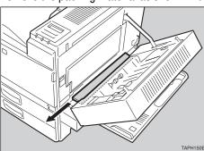
Open the right cover by pushing the catch upwards.
