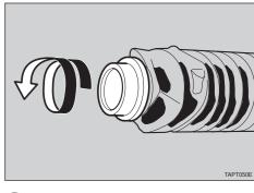
☐ After removing the black cap from the bottle, toner can scatter easily. Do not shake or jar the bottle.
