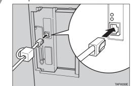
Connect the other side of the cable into the network. Secure Λ the cable.
