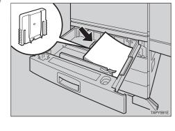
5 Slide the tray into the printer until it stops.
