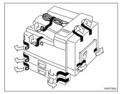
Open the bypass tray (1). And then open the duplex unit by pushing the catch upwards ((2)).
