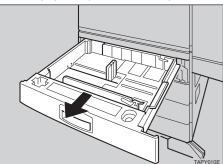
Pinch the sides of the rear guide (1), and remove it (2).
