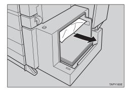
If you cannot remove the misfed paper in step **2**, close the top cover of the Large Capacity Tray RT36 and pull the lever (①) to extend the connecting unit (②).
