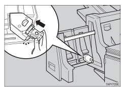
**7** Slide the stack unit into the Finisher SR720.
