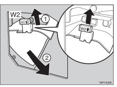
**5** Push the blue button W3 to open the cover (①), then remove the misfed paper (②).
