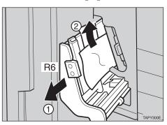
Return the stack unit to its original position (①) and close the front cover of the Finisher SR730 (②).
