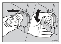
**7** Slide the stack unit into the Finisher SR730 (①), and close the cover (②).
