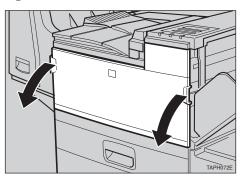
Turn the blue knob B counterclockwise (1) and remove the misfed paper from inside of the right cover (2).
