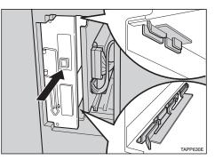
E Lock the printer board with the two screws you removed in step4.
