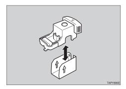
Add a new refill and align the arrows on the refill case and the cartridge, and push the refill case in until it clicks.
