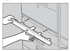
**6** Pull the second paper tray (Tray 2) up until it stops. After that, lift it slightly, then pull it out.
