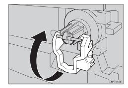
**3** While pushing the green lever to the right (①), hold the handle and gently slide the toner holder out (②).
