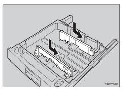
**1** Lock the side guides with the four screws you removed in step **4**.
