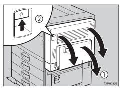
**2** Open the cover Z1 to the left (①), and remove the misfed paper (②).
