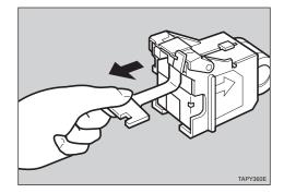
**6** Reinstall the cartridge, and press down on the cartridge until it clicks into place.
