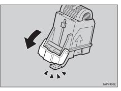
**6** Reinstall the cartridge, and press the cartridge down until it clicks into place.
