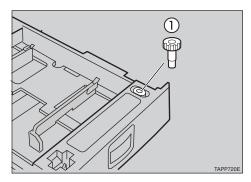
Remove the four screws inside of the tray you removed in step **1**.
