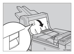
If you cannot remove the misfed paper in step **2**, remove the misfed paper (**1**) while pushing the blue lever R2 downwards in a clockwise direction (**2**).
