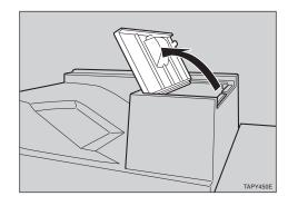
Pull the blue lever W5 to the right to open the cover (①), then remove the misfed paper (②).
