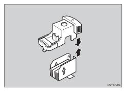
**5** Pull out the ribbon from the bottom of the refill case.
