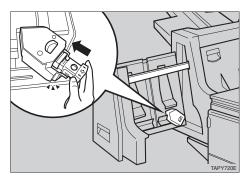
**2** Slide the stack unit into the Finisher SR720.
