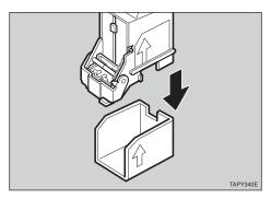
Add a new refill and align the arrows on the refill case and the cartridge, and push the refill case in until it clicks.
