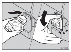
**2** Slide the stack unit into the Finisher SR730 (①), and close the cover (②).
