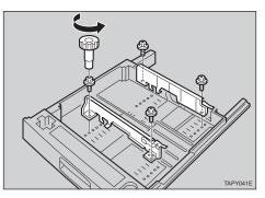
**E** Re-position the side guide to hold the paper size you want to load.
