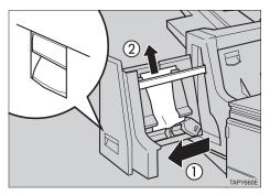
**6** Slide the stack unit into the Finisher SR720 until it stops.
