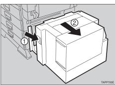
Remove the misfed paper from the left side of the Large Capacity Tray RT36.
