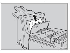
While pushing the blue lever R3 upwards in a clockwise direction (①), remove the misfed paper (②).
