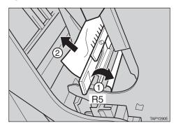
Hold the blue lever R6 and pull out the stack unit (①), then remove the misfed paper (②).
