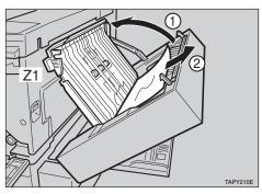
**1** If you cannot remove the misfed paper in step **2**, remove it (2) while opening the cover Z2 to the left (1).
