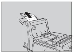
2 While pushing the blue lever R1 upwards (①), remove the misfed paper (②).
