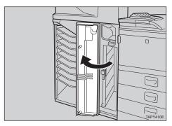
Push the blue lever W1 downwards to open the cover inside (①). Then remove the misfed paper (②).
