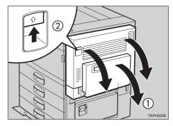
**2** Open the right cover by pushing the catch upwards.
