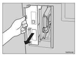
Confirm that the notch on the memory unit is on the right as shown in the illustration. Tilting the memory unit with the notch on the right, slide it into the slot as shown in the illustration (①). Then, move it upward until it clicks into place (②).
