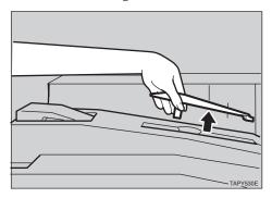
② Reinstall the guide in the opposite direction as shown in the illustration.
