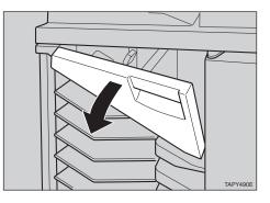
**E** Turn the blue lever W4 counterclockwise to open the cover (①), then remove the misfed paper (②).
