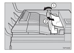
**2** Open the bypass tray (1). And then open the duplex unit by pushing the catch upwards (2).
