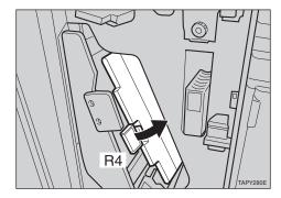
**7** If you cannot remove the misfed paper in step **6**, remove it (2) while pushing the blue lever R5 upwards in a clockwise direction (1).
