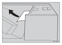
If your printer is equipped with both the Finisher SR730 and the Mailbox CS360, open the triangular cover on the front of the Mailbox CS360.
