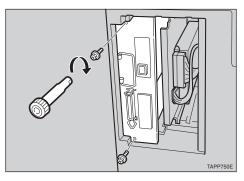
**2** Return the cover to its original position with the four screws you removed in step **2**.
