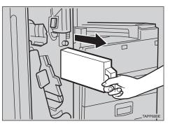
**B** Reinstall the punch waste box.
