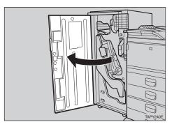
**2** Pull out the punch waste box and remove the paper chips.
