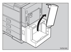
**B** Load paper with the long-edge side of the paper pressing against the printer side.
