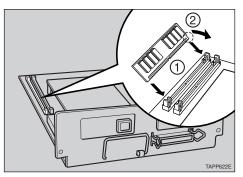
Align the printer board with the top and bottom rails in the printer, and then insert the printer board slowly until it clicks into place.
