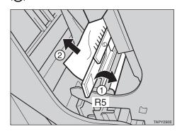
Hold the blue lever R6 and pull out the stack unit (1), then remove the misfed paper (2).
