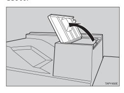
Pull the blue lever W5 to the right to open the cover (1), then remove the misfed paper (2).
