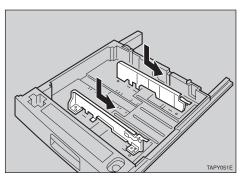
6 Lock the side guides with the four screws you removed in step 4.
