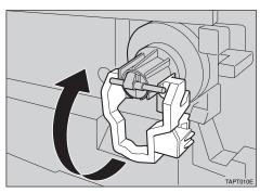
While pushing the green lever to the right (①), hold the handle and gently slide the toner holder out (②).
