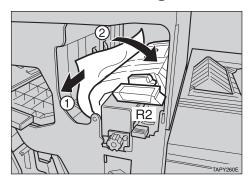
While pushing the blue lever R3 upwards in a clockwise direction (①), remove the misfed paper (②).
