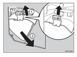
Push the blue button W3 to open the cover (1), then remove the misfed paper (2).
