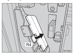
If you cannot remove the misfed paper in step **G**, remove it (②) while pushing the blue lever R5 upwards in a clockwise direction (①).
