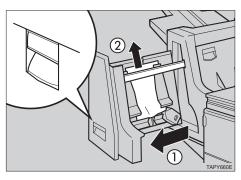
Slide the stack unit into the Finisher SR720 until it stops.
