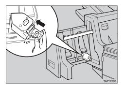
Slide the stack unit into the Finisher SR720.
