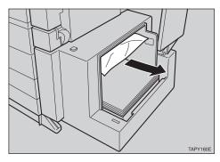
If you cannot remove the misfed paper in step **2**, close the top cover of the Large Capacity Tray RT36 and pull the lever (1) to extend the connecting unit (2).
