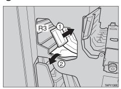
Push the lever R4 to the left (1) and remove the misfed paper (2).
