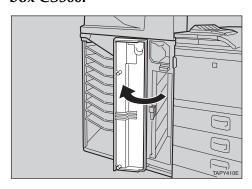
Push the blue lever W1 downwards to open the cover inside (1). Then remove the misfed paper (2).
