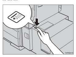
When the button stops blinking and is lit, open the top cover.
