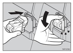
Slide the stack unit into the Finisher SR730 (①), and close the cover (②).
