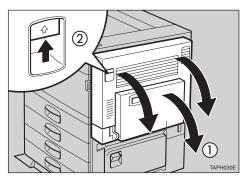
Open the cover Z1 to the left (①), and remove the misfed paper (②).
