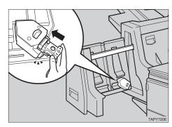
Slide the stack unit into the Finisher SR720.
