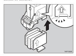
Pull out the ribbon from the bottom of the refill case.
