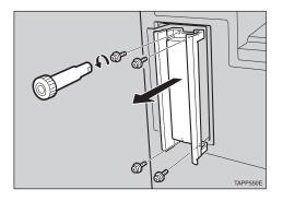
A Remove the two screws locking the printer board.
