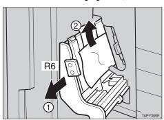
Return the stack unit to its original position (1) and close the front cover of the Finisher SR730 (2).
