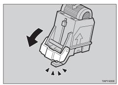
Reinstall the cartridge, and press the cartridge down until it clicks into place.
