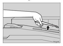
$\ensuremath{\mathfrak{D}}$  Reinstall the guide in the opposite direction as shown in the illustration.
