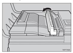
Remove the misfed paper by turning the blue knob C as shown in the illustration.
