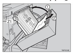
If you cannot remove the misfed paper in step 2, remove it (2) while opening the cover Z2 to the left (1).
