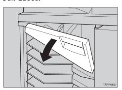
Turn the blue lever W4 counterclockwise to open the cover (1), then remove the misfed paper (2).
