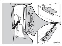
2 Lock the printer board with the two screws you removed in step 4.
