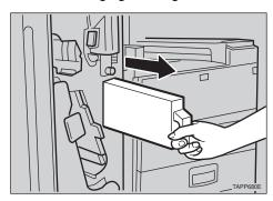
B Reinstall the punch waste box.
