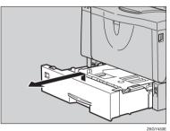
While lifting the front side of the tray, pull it out of the printer.
