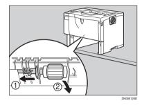
While sliding the green lock lever to the right (①), set the new roller
