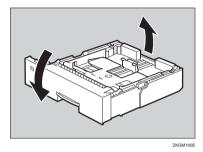
**5** Use a sharp-pointed item like a ball-point pen, to release the two catches that lock the friction pad.
