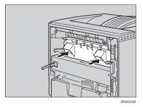
**5** Push the lock levers of the fusing unit down until it clicks.
