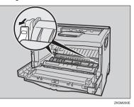
**5** Hold the green parts of the roller on both sides, and remove the roller from the printer as shown in the illustration.
