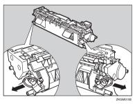
**5** Replace the new fusing unit into the printer.
