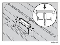
After pushing in the friction pad, try pushing it several times to check it is properly installed. If it jumps back into position due to the force of the spring, it is properly installed.
