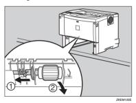
While sliding the green lock lever to the right (①), set the new roller (②). After that, return the green lock lever to its original position (③).
