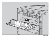
**2** Lift the lock levers of the fusing unit as shown in the illustration.
