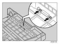
**5** Return the paper tray to its original position, and remove the friction pad from the tray.
