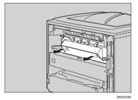
**4** Pull out the pins on both sides of the new fusing unit.
