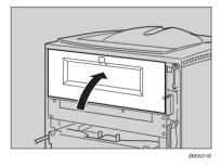
8 Reinstall the optional Duplex Unit if it was removed in step 1, "Replacing the Paper Feed Rollers".
