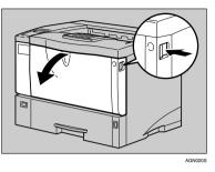
**2** Remove the fixing material inserted between toner cartridge and the printer.
