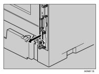
**4** Carefully insert the network data protection unit, until the card clicks into the place.
