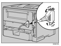
**B** Securely attach the other end of the parallel cable to your computer's parallel port. Secure the cable.
