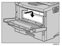
**2** Close the front cover by pressing the indentations on the left and right sides.
