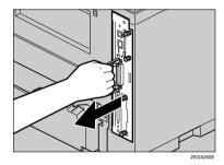
**2** Place the controller board on a flat surface.
