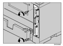
**4** Pull out the handle of the controller board.
