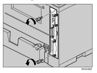
**5** Pull out the handle of the controller board.
