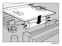
${f I}$  Fasten the network interface unit to the controller board with the two screws.
