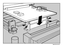
Fasten the 802.11b Interface Unit to the controller board with the two screws.
