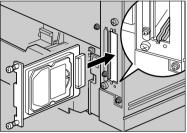
**5** Fasten the two screws (using a coin, etc.) to fix the hard disk drive.
