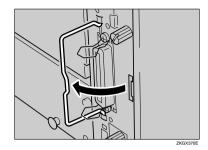
**5** Pull the handle, and then slide the controller board out.
