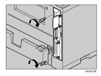
Attach the antenna cap to the card with the side that has both corners of the antenna cap cut out facing the screws.
