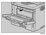
**B** Lift the front side of the toner cartridge, and then pull it out of the printer.
