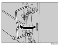
**6** Pull the handle, and then slide the controller board out.
