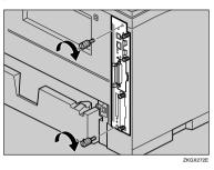
Align the power cable to the left side groove of the duplex unit, and then slide the duplex unit in until it is connected to the printer.
