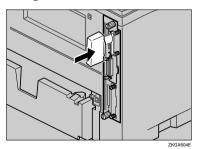
Align the power cable to the left side groove of the duplex unit, and then slide the duplex unit in until it is connected to the printer.
