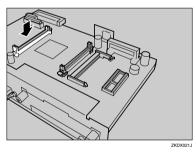
B Remove the default memory unit before installing a new memory unit. Press down the levers on both sides to remove the default memory unit.
