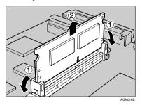
Align the notch of the memory unit to the slot, and then push it down until it clicks.
