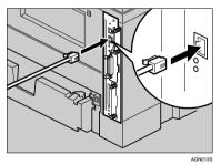
**B** Connect the other end of the cable to the printer's network, such as a hub.
