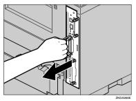
Place the controller board on a flat surface.
