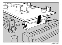
**D** Fasten the 1394 interface unit to the controller board.
