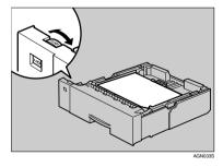
□ When loading paper other than A4 □ (short-edged feed) or 8<sup>1</sup>/<sub>2</sub> × 11 □ (short-edged feed), you should extend the tray.
