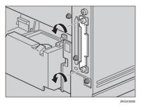
4 Slowly insert the Hard Disk Drive while aligning it with the top and bottom rails in the printer until it stops.
