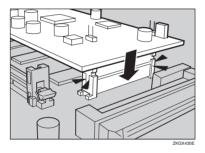
Fasten the 1394 Interface Unit to the controller board.
