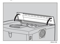
5 Holding the Mailbox on both sides, align the catches with the holes on the printer and insert.
