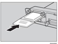
Match the controller board to the top and bottom rail using the "▼" mark, and then slide it into the printer slowly until it stops.
