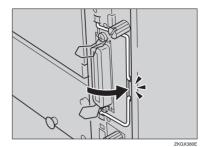
Fasten the controller board to the printer with the two screws.
