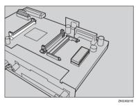
9 Insert the Memory unit to the slot by placing the notch of the unit to the projection of the slot, and then push it down until it clicks.
