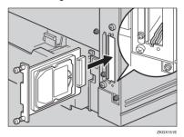
**5** Fasten the two screws (using a coin, etc.) to fix the Hard Disk Drive.
