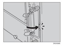
**B** Fasten the controller board to the printer with the two screws.
