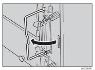
**6** Pull the handle and slide the controller board out.
