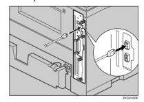
**2** Connect the other end of the 1394 interface cable to the computer or the other IEEE 1394 node.
