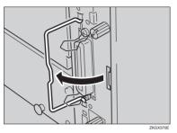
**5** Pull the handle and slide the controller board out.
