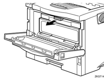
3 While lifting the front side of the toner cartridge, pull it out of the printer.
