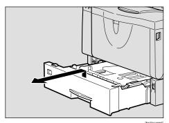
3 While lifting the front side of the tray, pull it out of the printer.
