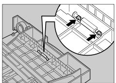
6 Return the paper tray to its original position, and remove the friction pad from the tray.
