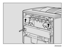
**3** Pull the fusing unit out.
