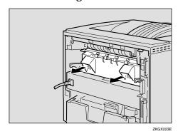
While holding the tab, remove the misfed paper.
