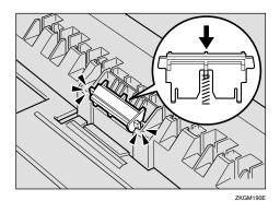
After pushing in the friction pad, try pushing it several times to check it is properly installed. If it jumps back into position due to the force of the spring, it is properly installed.
