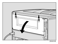
**2** Remove the rear cover in a horizontal direction.
