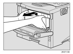
Wipe around the metallic registration roller by turning with a soft damp cloth.
