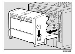
2 Push the under board levers (1) and pull the Duplex Unit out of the printer (2).
