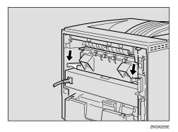
Insert the rear cover to the inside grooves on both sides of the printer in a horizontal direction.
