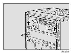
**7** Pull the fusing unit out.
