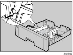
While pinching the rear guide, slide it along the edge of the envelope stack.
