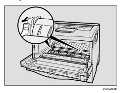
5 Hold the green parts of the roller on both sides, and remove the roller from the printer as shown in the illustration.
