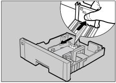
8 Lift the front of the tray, and slide it carefully into the printer until it stops.
