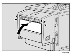
4 While lifting the lever (1), open the cover of the Duplex Unit (2).
