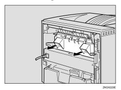
Pull out the pins on both sides of the new fusing unit.
