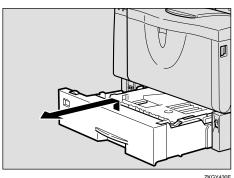
2 While lifting the front side of the tray, pull it out of the printer.
