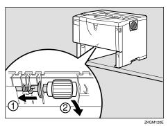
4 While sliding the green lock lever to the right (1), set the new roller (2). After that, return the green lock lever to its original position (3).
