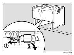
Wipe the rubber part of the roller with a soft damp cloth. After that, wipe it with a dry cloth to remove the water.
