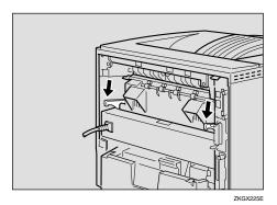
**7** Reinstall the rear cover removed in step **1**.
