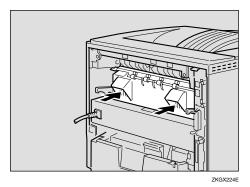
6 Push the lock levers of the fusing unit down until it clicks.
