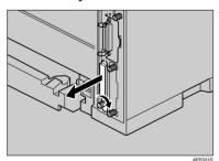
Carefully insert the network data protection unit, until the card clicks into the place.
