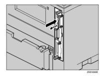
Attach the antenna cap to the card with the side that has both corners of the antenna are cut out facing the screws.
