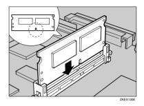
For network standard model printer, remove the default SDRAM module before installing a new SDRAM module. Press down the levers on both sides to remove the default memory unit.
