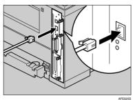
Connect the other end of the cable to the printer's network, such as a hub.
