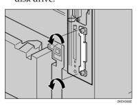
Slowly insert the hard disk drive while aligning it with the top and bottom rails in the printer until it stops.
