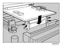
Pasten the Bluetooth interface unit to the controller board with the two screws.
