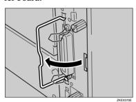
Pull the handle, and then slide the controller board out.
