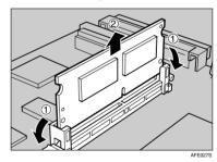
Align the notch of the SDRAM module to the slot, and then push it down until it clicks.
