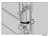
Fasten the controller board to the printer with the two screws.
