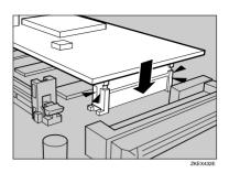
**9** Fasten the network interface board to the controller board.
