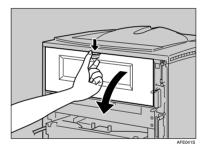
Remove the rear cover in the horizontal direction.
