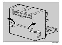
Place a finger in the printer's rear cover finger-hole (upper center) and pull it open.
