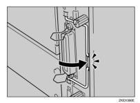
11 Fasten the controller board to the printer with the two screws.
