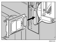
Fasten the two screws (using a coin, etc.) to fix the hard disk drive.
