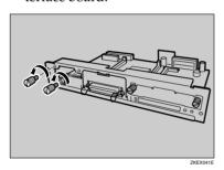
Attach the network interface board to the controller board.
