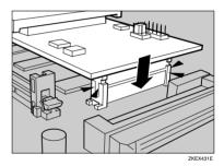
Fasten the 802.11b interface unit to the controller board with the two screws.
