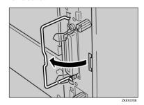
Holding the handle, slowly pull out the controller board.
