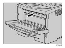
**E** Lift the front side of the toner cartridge, and then pull it out of the printer.
