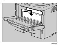
Close the front cover by pressing the indentations on the left and right sides.
