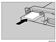
Match the controller board to the top and bottom rail using the "▼" mark, and then slide it into the printer slowly until it stops.
