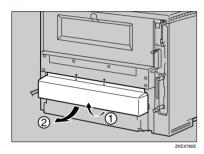
Push in the duplex unit along the rails at the back of the printer.
