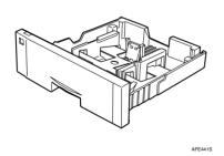
Pull out the second paper tray (Tray 2) of the optional paper feed unit until it stops. After that, lift it slightly, and then pull it out.
