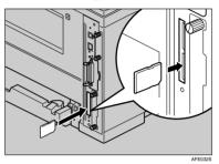
Reattach the cover over the network data protection unit. Fasten the screw to secure the cover.
