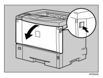
2 Remove the fixing material inserted between toner cartridge and the printer.
