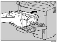
Insert the toner cartridge in its appropriate position by gently pushing down.
