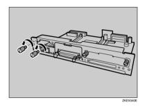
Attach the 1394 interface unit to the controller board.
