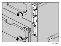
Pull out the handle of the controller board.
