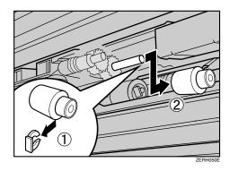
Remove the stopper from the paper feed roller C (1), and then remove the roller (2).
