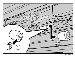
Hold the new paper feed roller C with its gear towards the shaft. Insert it into the rear shaft so that the roller gear interlocks with the shaft gear (1). Lock the roller with the stopper (2).
