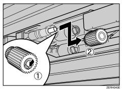
Remove the stopper from the paper feed roller B (1), and then remove the roller (2).
