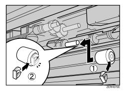
Hold the new paper feed roller B with its gear towards the shaft. Insert it into the rear shaft so that the roller gear interlocks with the shaft gear (1). Lock the roller with the stopper (2).
