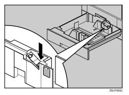
**3** Align all four sides of the paper stack, and then load it in the tray.
