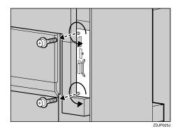
The removed screws will be used later to fasten the Controller Board. **3** Holding the handle, pull out the Controller Board slowly.
