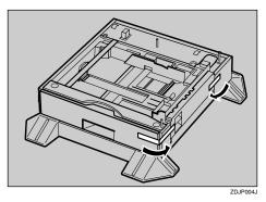
Adjust the four corners of the printer to those of the 500-sheet Paper Feed Unit, and then lower the printer slowly into place.
