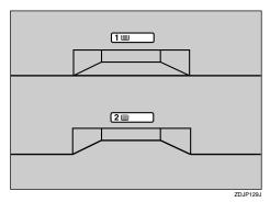
A sticker, stating that paper for an ink-jet printer cannot be used with this printer, is supplied. Please attach the sticker to the bottom right corner of the top of the printer [A] so that sticker is easy to see.
