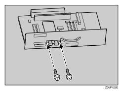
9 Insert the Controller Board into the top and bottom rails, and slide it in slowly until it stops.
