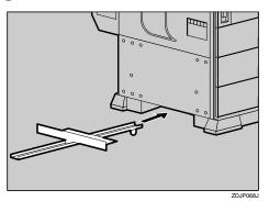
8 Hook the hole of the mounting bracket on the screw that was temporarily fastened in step 5.
