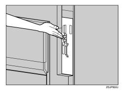
Tighten two screws to fasten the Controller Board back into its original position using provided screwdriver.
