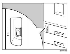
2 Connect the power cable to the connector on the back of the printer.
