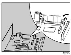
**6** Adjust the notch of the Memory Unit to the slot and insert vertically.
