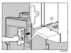
Insert the Controller Board firmly by pushing the left area as shown in the illustration.
