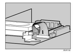
Connect the power cable to the Controller Board.
