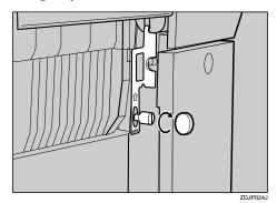
Close the right cover of the 2000sheet Large Capacity Tray. Stick label "3" above the handle on the front of the 2000-sheet Large Capacity Tray.
