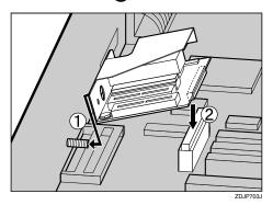
Confirm that the User Account Enhance Unit is connected firmly to the Controller Board.
