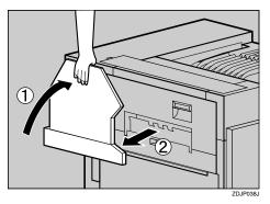
Remove the two small covers on the upper left cover of the printer.
