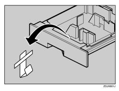
**5** Take out the packaged items, making sure there are two thumb screws and one mounting bracket. Close the tray of the 500-sheet Paper Feed Unit tightly.
