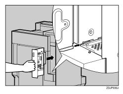
Insert the Controller Board firmly by pushing the left area as shown in the illustration.
