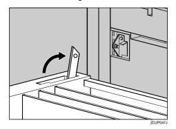
4 Hook the hole of the auxiliary bar on the mounting bracket of the printer.
