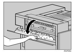
Pinch the two small covers and pull in the direction of the arrow to remove them.
