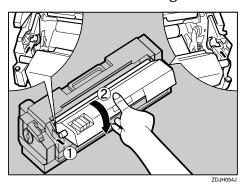
8 Holding the green handle with one hand, use your other hand to push the front area of the handle to a slight slant, and then push the Fusing Unit slowly to the back.
