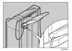
With the 2 Tray Fisher Tray laid horizontally, slide it in at a slant until it stops.
