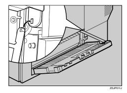
Fasten the bracket with the other thumb screw. Use a coin to fasten it tightly.
