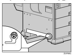
9 Holding the mounting bracket with both hands, move it in the direction of up (1)  $\Rightarrow$  right (2).
