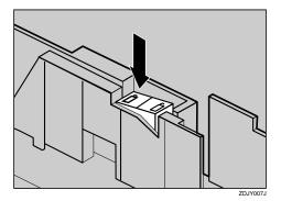
**6** Gripping both edges of the end guide (**1**), move it to the position of the loaded paper (**2**).
