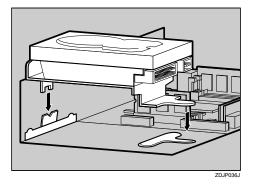
**7** Tighten two screws to fasten the Printer Hard Disk to the Controller Board using provided screwdriver.
