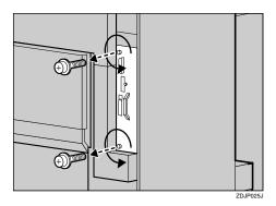
The removed screws will be used later to fasten the Controller Board.
