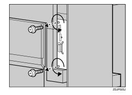
The removed screws will be used later to fasten the Controller Board.
