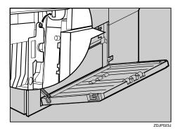
D Fasten the bracket with the other thumb screw. Use a coin to fasten it tightly.
