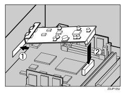
Confirm that the 1394 Interface Unit is connected firmly to the Controller Board.
