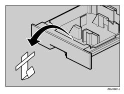
**5** Take out the packaged items, making sure there are two thumb screws and one mounting bracket. Close the tray of the 1000-sheet Paper Feed Unit tightly.
