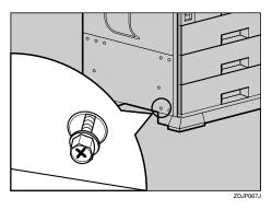
Insert the rail, assembled in stepinto the bottom area of the printer.
