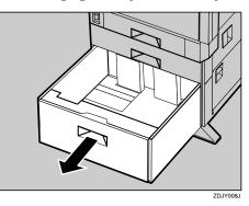
**2** Align all four sides of the paper stack, and then load two stacks next to each other.
