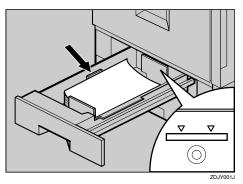
**2** Align all four sides of the paper stack, and then load it in the tray.
