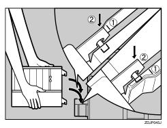
The hooks of the Duplex Reversal Unit grasp the bar inside the groove of the stand.
