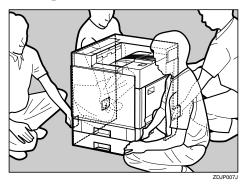
Take out the packaged items, making sure there are two thumb screws and one mounting bracket. Close the tray of the 2000-sheet Large Capacity Tray tightly.
