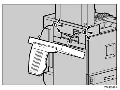
**B** Remove the adhesive tape of the cable of the 4-bin Mailbox.
