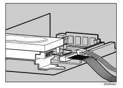
**9** Connect the flat cable to the Controller Board.
