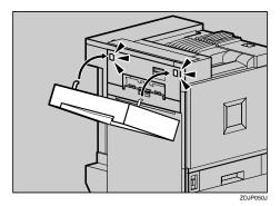
**7** Remove the adhesive tape which hold the cable, and then connect the cable of the Duplex Reversal Unit to the upper connector on the back of the printer.
