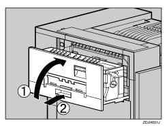
Attach the External Tray to the printer. Insert the hooks of the External Tray into the printer slits, and then lower it toward you.
