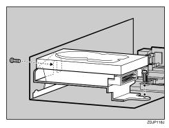
8 Connect the power cable and flat cable to the Printer Hard Disk.
