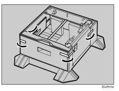
Adjust the four corners of the printer to those of the 2000-sheet Large Capacity Tray, and then lower the printer slowly into place.
