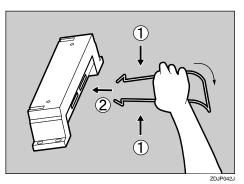
8 Insert the claws of the stand into the holes on the left side of the printer (1), and push down (2).
