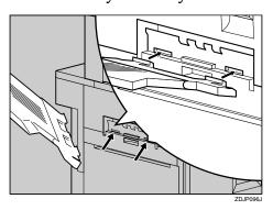
If the Duplex Unit is installed, return the Duplex Reversal Unit to its original position. Lift it slowly until you hear a click.
