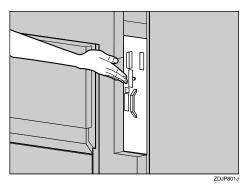
**9** Tighten two screws to fasten the Controller Board back into its original position using provided screwdriver.
