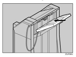
**3** Fasten the Fisher Tray with a short screw using provided screwdriver.
