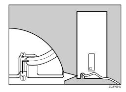
Connect the cable of the 4-bin Mailbox to the lower connector on the back of the printer.
