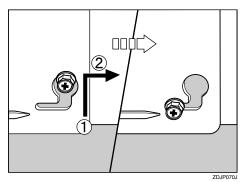
With the left corner of the mounting bracket adjusted to the position shown by the arrow in the illustration, fasten the left side of the mounting bracket with a long screw using provided screwdriver. Also tighten the screw on the right side that was temporarily fastened in step **G**.
