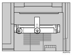
**B** Fasten the right side of the connecting bracket with a long screw using provided screwdriver. Also tighten two screws that were temporarily tightened in step **1**.
