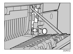
Close the right cover of the 500sheet Paper Feed Unit. Stick label "3" above the handle on the front of the 500-sheet Paper Feed Unit.
