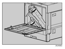
Remove the securing pin, as shown in the illustration, from the Transfer Unit. Pinch it, and then pull it out.
