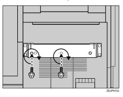
Hook the connecting bracket on the screws that were temporarily tightened in step **1**.
