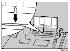
**7** Keep pressing the Memory Unit down until it clicks into the locked position.
