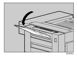
Installing the Duplex Feed Unit
