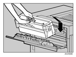
Confirm that the Fusing Unit is set to the printer vertically.
