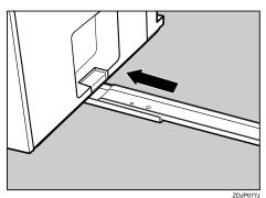
**1** Fasten the rails with a long screw using provided screwdriver.
