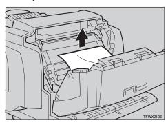
When the misfed paper is in the main section of the photoconductor unit, turn the dial downward then remove the misfed paper in the printer.
