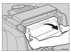
Hold the inset grips (green part) of the photoconductor unit, remove the photoconductor unit from the printer, and place it carefully inside the new photoconductor unit's box.
