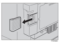
2 Remove the ozone filter from inside the ventilator hole cover.
