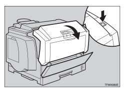
Turn the dial downward, then remove the misfed paper in the printer.
