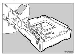
If installing two paper feed units, place one paper feed unit on the other paper feed unit at first. If installing only one paper feed unit, go to step 2.
