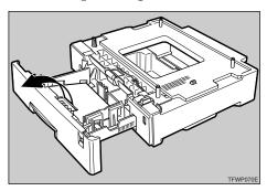
Remove the ring attached to the red tag.
