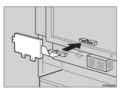
Set the hard disk in the lower left corner at the rear of the printer, as shown in the illustration. Make sure that the screw holes of the hard disk align with the screw holes of the printer. And fasten it with the screws that are enclosed in the box using the screw driver.
