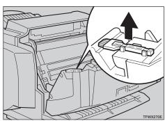
Insert the cleaning brush into the back of the guide (light blue) until it stops, and then move it left and right 4 or 5 times.
