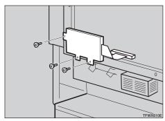
Attach the back plate to its original position, and fasten it with screws that were removed in step **3**.
