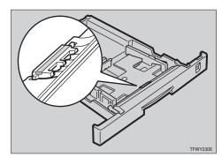
2 Load paper with the print side up into the paper tray. While lifting the front side of the tray, insert the paper tray into the printer. Then push in until it stops.
