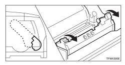
Hold the inset grips (green part) of the new photoconductor unit, and insert the photoconductor unit into the photoconductor unit holder.
