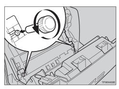
6 Hold the inset grips (green part) of the photoconductor unit, and pull the top side of the photoconductor unit forward.
