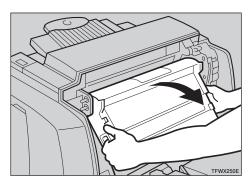
Remove the cleaning brush from back of the front cover.
