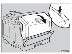
Hold the inset grips (green part) of the photoconductor unit, and pull the top side of the photoconductor unit forward.
