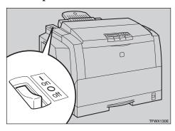
After turning on the printer, it takes about eight minutes to warm up before being able to print.
