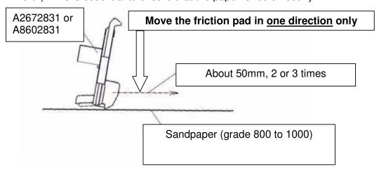
After smoothing out the pad surface, check the paper feed with a full paper tray.
