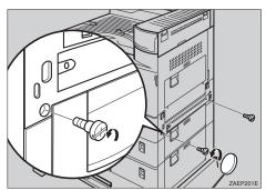
Remove the two socket screws holding the cover on the right side of the printer using the included wrench, and remove the cover.
