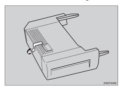
If you installed the duplex unit, open the duplex unit by lifting the catch.
