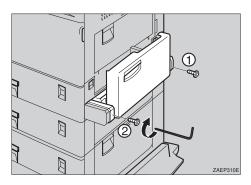
Remove the adhesive tape holding the bypass tray and cable, and attach the connector to the socket on the left bottom side of the back of the printer.
