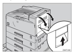
Open the upper right cover by lifting the handle.
