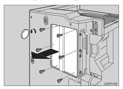
Tilt the memory unit so that it is 30 degrees perpendicular to the slot (1), and push it forward (2). It should make click into place.
