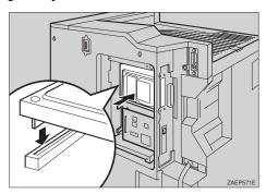
**6** Fasten the two screws that were removed in step **6** to attach the hard disk to the printer.
