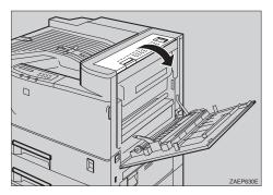
Press the upper right cover in the direction as shown in the illustration (1), and remove the upper right cover (2).
