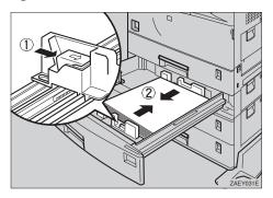
6 Set the paper guide lock to the "locked" position.
