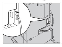
Push the cable of the connected harness into the groove for the cable until it stops.
