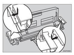
Slide the bypass tray into the printer aligning the grooves of the right and left sides of the bypass tray onto the rails inside the holder.
