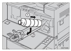
Slide the toner holder into the printer until it clicks into place, and push the green handle down.
