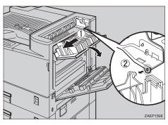
Use a coin to remove the screw from the upper cover of the printer.
