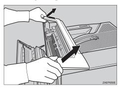
Remove the interchange unit cover from the interchange unit.
