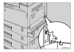
Lower the duplex unit so that the groove in each arm of the unit forms a joint with the pin inside the holder as shown in the illustration.
