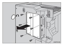
4 Use a coin to remove the two screws, and remove the cover.
