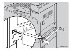
Use the wrench to fasten the four socket screws in the order shown in the illustration (1 - 4), to secure the holder to the printer.
