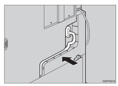
Attach cover 1 (1) and secure cover 1 to the printer fastening the screw (2).
