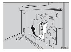
While pushing the green lever (1), hold the handle and slide the toner holder out slightly (2).
