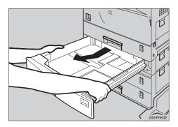
Use a coin to fasten the two screws that join the paper feed unit and the printer.
