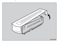
Move the cable to the back of the printer. Place the interchange unit onto the printer as shown in the illustration.
