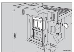
Attach the printer board cover that was removed in step **E**, and use a coin to fasten the six screws.
