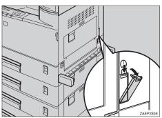
Mount the brackets in the holes inside of the cover that was opened in step 2. Use the wrench to fasten the socket screw, to secure the hook to the printer.
