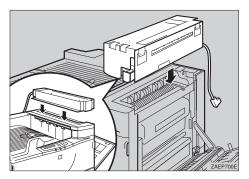
Open the upper right cover (1) and slide the interchange unit while keeping the cover perpendicular to the printer (2). At this time, confirm that the projection (3) is placed in the hole securely as shown in the illustration.
