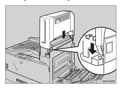
Fasten the two screws by hand and secure the mailbox to the printer. Use a coin to fasten the screws securely.
