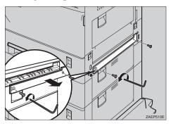
Mount the brackets of the holder by placing them in the printer and pushing downwards slightly.
