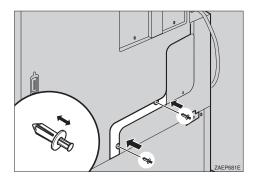
Turn the adjuster at the center bottom of the paper feed unit clockwise until it touches the floor.
