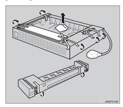
A Remove the two small covers from the top right side of the printer.
