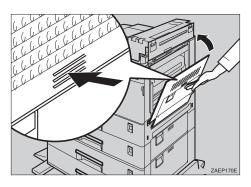
If the mailbox is not installed, attach the interchange unit cover that was removed in step 2. Attach the side of the cover facing the front of the printer first (1) and then the other side of the cover (2).
