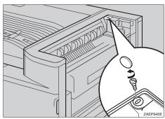
Put your fingers inside the upper cover of the printer and remove the cover by pulling upward.
