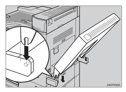
Hang the support bar in the duplex unit on to the hook that was attached in step (1), and secure the bar by attaching the holder to the joint (2).
