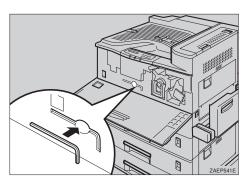
☐ After installed the last option that you want, print a configuration page to confirm the installation. If the new device is listed in the column of configuration options, then it has been properly installed. For more information on printing a configuration page, see P.37 "Printing a Configuration Page".
