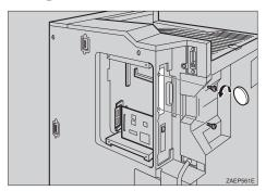
Align the hard disk interface connector over the printer interface port, and push gently but firmly on the hard disk until it is completely connected.
