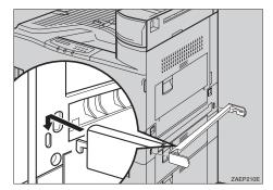
Use the wrench to fasten the four socket screws in the order as shown in the illustration (1) - (4), to secure the holder to the printer.
