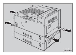
By holding the handles, align the front face of the printer and the paper feed unit, then place the printer on the paper feed unit.
