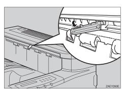
Put the paper size seal directly below the paper size display of the front on the paper tray.
