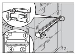
Remove the small cover on the right side of the printer.
