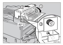
Fasten the two screws with fingers, while keeping the upper right cover of the interchange unit perpendicular to the printer, and secure the interchange unit to the printer. Use a coin to fasten the screws.
