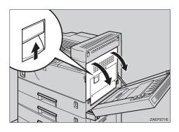
If the cover of the interchange unit is attached, remove it by sliding it out toward the back of the printer.
