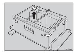
Slide out the four handles on both sides of the printer.
