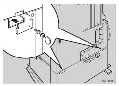
Remove the adhesive tape holding the cable and connect the harness on the back of the printer.
