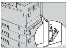
Mount the brackets in the holes inside of the cover that was opened in step **2**. Use the wrench to fasten the socket screw, to secure the hook to the printer.
