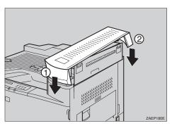
Attach the connector of the interchange unit to the socket on the back of the printer as shown in the illustration.
