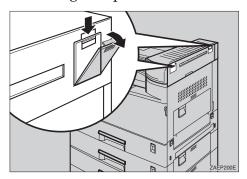
Use a coin to remove the two screws on the right side of the printer.
