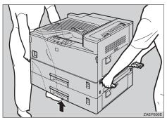
☐ Do not pinch the harness on the back of the paper feed unit and the printer.
