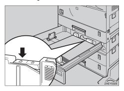
Align the rear guide for the loaded paper size slightly by pushing the releasing lever of the rear guide.
