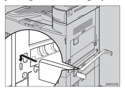
Use the wrench to fasten the four socket screws in the order shown in the illustration (1) - (4), to secure the holder to the printer.
