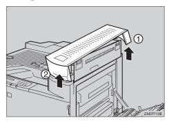
**7** Hold the mailbox on both sides and insert it into the printer from the top side of the printer.
