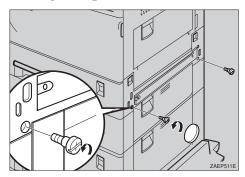
Use the wrench to remove the two socket screws from the cover on the right side of the printer, and remove the cover.
