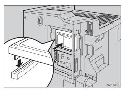
**6** Fasten the two screws that were removed in step **6** to attach the hard disk to the printer.
