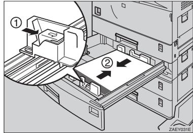
**6** Set the paper guide lock to the "locked" position.
