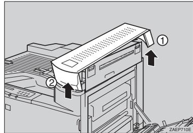
**7** Hold the mailbox on both sides and insert it into the printer from the top side of the printer.
