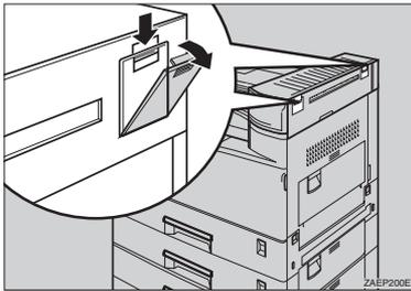
**5** Use a coin to remove the two screws on the right side of the printer.
