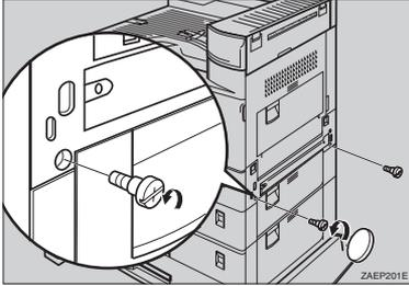
**5** Remove the two socket screws holding the cover on the right side of the printer using the included wrench, and remove the cover.
