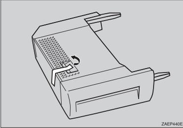
**4** If the duplex unit is already installed, open the duplex unit by lifting the catch.
