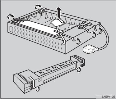
**4** Remove the two small covers from the top right side of the printer.
