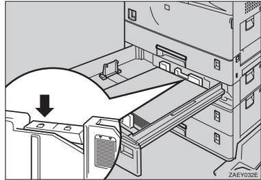
**7** Align the rear guide for the loaded paper size slightly by pushing the releasing lever of the rear guide.
