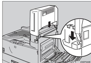
**8** Fasten the two screws by hand and secure the mailbox to the printer. Use a coin to fasten the screws securely.
