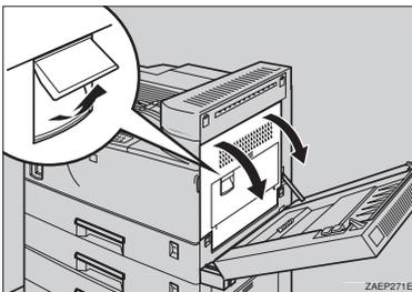
**6** If the cover of the interchange unit is attached, remove it by sliding it out toward the back of the printer.
