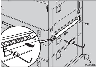
**6** Mount the brackets of the holder by placing them in the printer and pushing downwards slightly.
