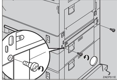
**6** Use the wrench to remove the two socket screws from the cover on the right side of the printer, and remove the cover.
