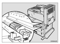
Raise slightly and pull the green lever attached to the paper feed rollers inside the printer on the lower right side.
