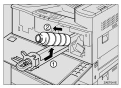
Move the new toner bottle back and forth about five or six times (①), and remove the black cap of the new toner bottle by turning it counterclockwise (②).
