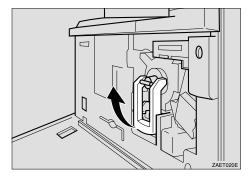
While pushing the green lever (1), hold the handle and slide the toner holder out slightly (2).
