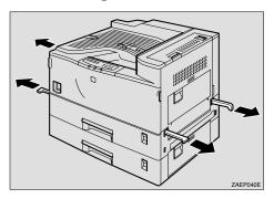
By holding the handles, lift the printer. The printer should be held by at least two people.
