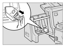
**2** Remove the empty refill case as shown in the illustration.
