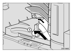
Close the covers in the following order: the right cover of the bridge unit, the upper cover of the interchange unit, the right cover of the printer, and the duplex unit.
