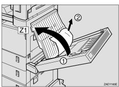
If the misfed paper was not removed in step 2, while lifting the lever, lift cover Z2 (1), and remove the misfed paper (2).
