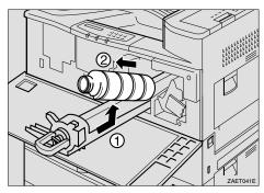
Move the new toner bottle back and forth about five or six times (1), and remove the black cap of the new toner bottle by turning it counterclockwise (2).
