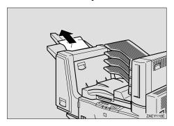
2 If the misfed paper was not removed in step 1, open the right cover of the finisher.
