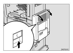
While lifting the lever, lift cover Z1 (1), and remove the misfed paper (2).
