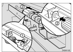
Check the motion of the paper feed roller to confirm that it is properly set.
