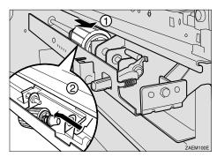
Wipe the rubber of the paper feed roller with a dry cloth.
