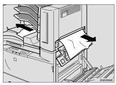
If the misfed paper was not removed in step **B**, open the upper cover of the bridge unit (1), and remove the misfed paper (2).
