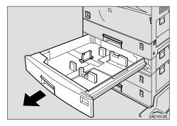
2 Set the paper guide lock to the "unlocked" position.
