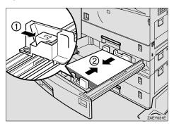
Set the paper guide lock to the "locked" position.
