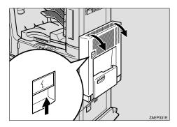
2 Open the right cover by lifting the catch (1), and open the upper cover of the interchange unit by pulling the handle (2).
