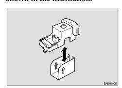
Align the arrows on the new refill case and the cartridge, and push the new refill case in until it clicks.
