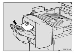
2 If the misfed paper was not removed in step 1, open the upper cover of the finisher (1) and remove the misfed paper (2).
