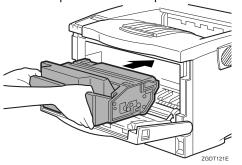
Insert the toner cartridge in its appropriate position by gently pushing down.
