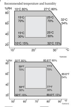
Possible operation range Recommended range The machine must be level within 5 mm, 0.2" both front to rear and left to right.
