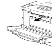
While lifting the front side of the toner cartridge, pull it out of the printer.
