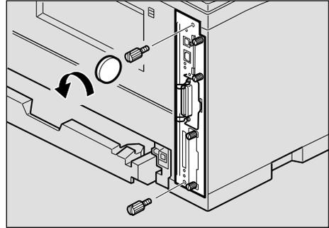
**5** Pull out the handle of the controller board.
