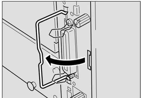
**6** Pull the handle and slide the controller board out.
