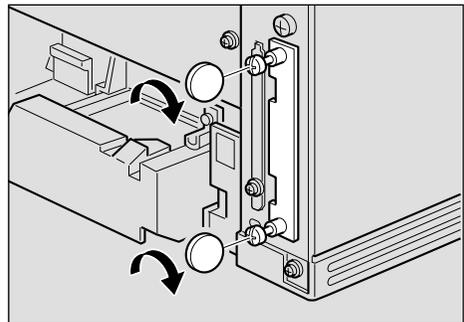
**6** Attach the interface cable to the printer.
