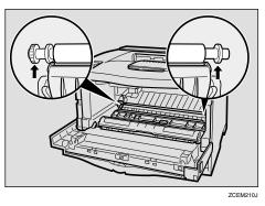
**6** Insert the new transfer roller on the socket with the gear of the roller positioned on the left.
