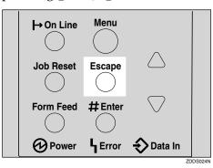
□ After making the printer settings, press **[On Line]** to return to the "Ready" condition.
