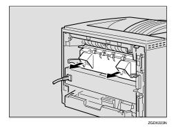
8 While holding the tab, remove the misfed paper.
