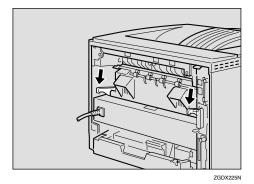
**1** Insert the rear cover to the inside grooves on both sides of the printer in a horizontal direction.
