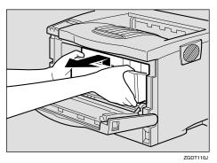
**3** Wipe around the metallic registration roller by turning with a soft damp cloth.
