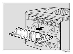
**6** Lift the lock levers of the fusing unit as shown in the illustration.
