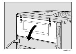
2 Remove the rear cover in a horizontal direction.
