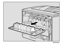
**2** Lift the lock levers of the fusing unit as shown in the illustration.
