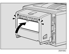
While lifting the lever (①), open the cover of the Duplex Unit (②).
