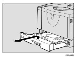
**2** While lifting the front side of the tray, pull it out of the printer.
