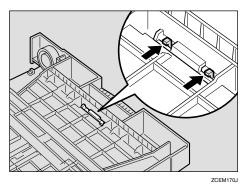
6 Return the paper tray to its original position, and remove the friction pad from the tray.
