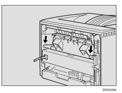
**6** Insert the rear cover to the inside grooves on both sides of the printer in a horizontal direction.
