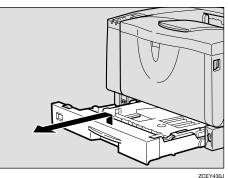
**3** While lifting the front side of the tray, pull it out of the printer.
