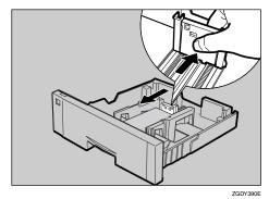
8 While lifting the front of the tray, place it into the printer. Then slide it until it stops.
