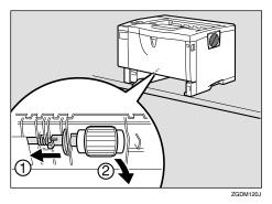
**6** Wipe the rubber part of the roller with a soft damp cloth. After that, wipe it with a dry cloth to remove the water.
