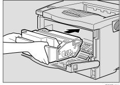
9 Push down the toner cartridge to insert it in its appropriate position.
