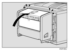
**2** Pull the Duplex Unit out of the printer until it stops, and remove the misfed paper.
