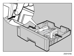
**7** While pinching the rear guide, slide it along the edge of the envelope stack.
