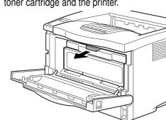
While lifting the front side of the toner cartridge, pull it out of the printer.
