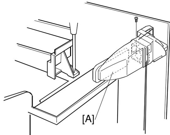
**NOTE:** Open the fan case (unhook at one location), and remove the fan motor (the interlock switch top is also removed.)
