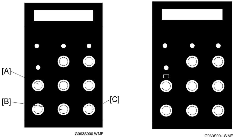
1. Turn the power switch on while holding the [Menu] [A], [Enter] [B] and [▼] [C] keys.
