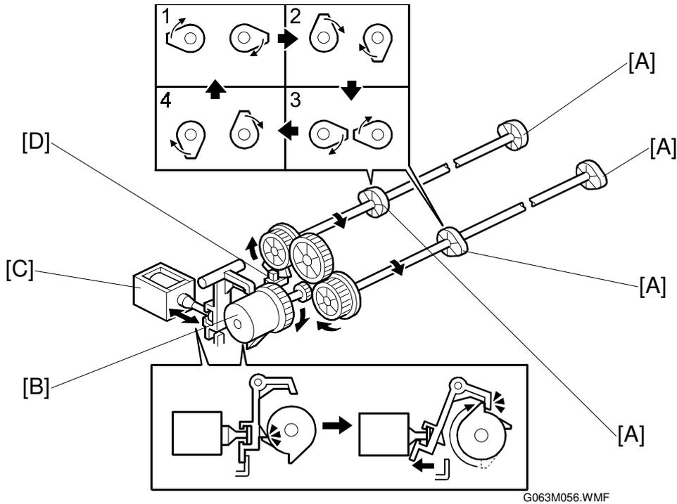
When the printer is idle, none of the toner cartridges contacts the OPC belt. During printing, the machine moves the toner cartridges into contact with the belt one at a time, in the order K, C, M, Y.
