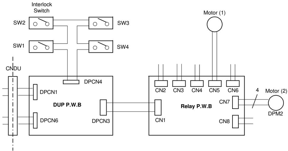
Defective duplex unit motor (1) or (2).
