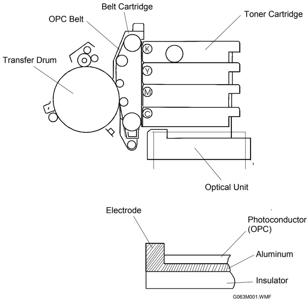
The OPC belt consists of a surface layer of organic photoconductor (OPC), an inner layer of insulation (PET), and an aluminum layer in between the two.
