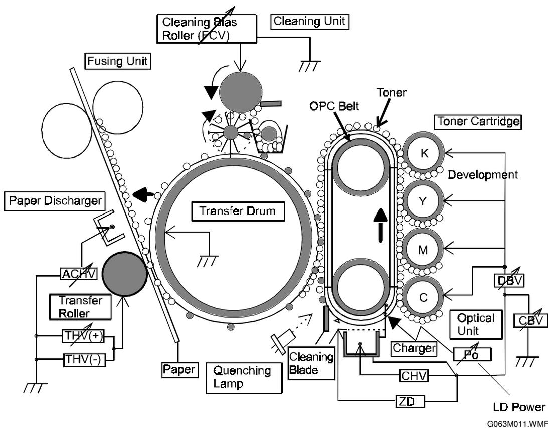
In the above diagram, blocks with a diagonal arrow through them indicate a power output that can be adjusted using an engine service mode. Potentiometers on the high voltage unit or laser diode drive board PCBs should not be touched.
