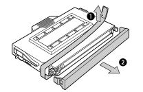
Align the toner cartridge (cyan) to the "C" mark of the printer as shown in the illustration. Slide the cartridge in along the printer's guide rail.
