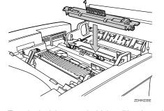
Turn the lock levers to hold the oil bottle and fuser cleaner
