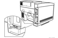
Check that the printer's power switch is set to the Off position (not depressed).
