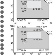
Possible operation range Recommended range The machine must be level within 5 mm, 0.2" both front to rear
