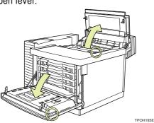
Lift the green lock levers to a vertical position.
