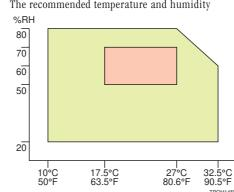
Possible operation range Recommended range The machine must be level within 5 mm, 0.2" both front to rear and left to right. To avoid possible build-up of ozone, make sure to locate this machine in a large well ventilated room that has an air turnover more than 30m<sup>3</sup>/hr/person.
