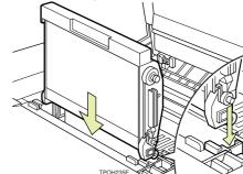
☐ When inserting the photoconductor unit, be careful not to touch or damege the surface.
