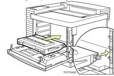
$\Box$  Do not use excessive force in sliding in the cartridge.
