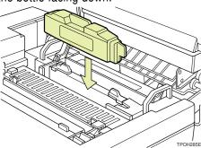
Install the fuser cleaner. When installing, the roller should be facing toward you.
