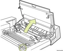
Remove the orange lock pins.
