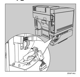
Connect the paper feed unit cable to the lower socket inside the printer securely. Make sure the protruding part of the cable connector is facing downward.
