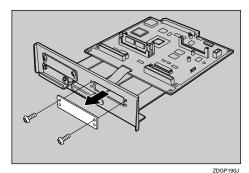
Insert the network interface board into the slot and fasten it with both screws that were removed in step [], as shown in the illustration.
