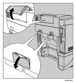
**4** Remove the two covers from the paper feed unit as shown in the illustration.
