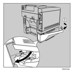
Confirm the location of the two guide pins and two hooks on the duplex unit, as well as the corresponding cutouts and holes on the paper feed unit and the printer.
