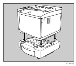
Set the locking plate, which was moved to the "RELEASE" position in step, to the "LOCK" position again.
