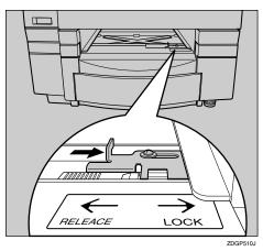
Insert the securing bracket removed in step [] into the groove under the printer, and secure the bracket using the screw removed in step [].
