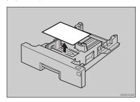
Remove the red protective sheet taped on the guide. Insert the paper tray into the printer until it stops.
