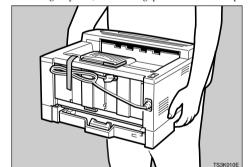
Remove the five pieces of adhesive tape from the printer as shown in the illustration.
