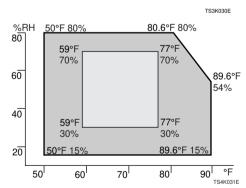
Possible operation range Recommended range The machine must be level within 5 mm, 0.2" both front to rear
