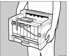
Remove the five pieces of adhesive tape from the printer as shown in the illustration.
