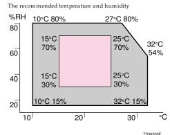
Possible operation range Recommended range The machine must be level within 5 mm, 0.2" both front to right
