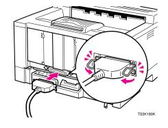
Attach the other end of the interface cable to the interface connector of the computer. Secure the cable.
