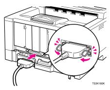
Attach the other end of the interface cable to the interface connector of the computer. Secure the cable.
