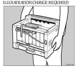
Remove the four pieces of adhesive tape from the printer as shown in the illustration.
