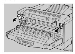
2 Slide the fusing unit toward you (①), and remove it from the printer (②) as shown in the illustration.
