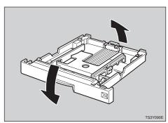
Release the two black catches, that lock the friction pad, using a the holes of the paper tray as
