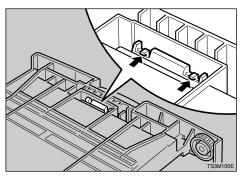
Turn the paper tray to the original position, and remove the friction pad from the tray.
